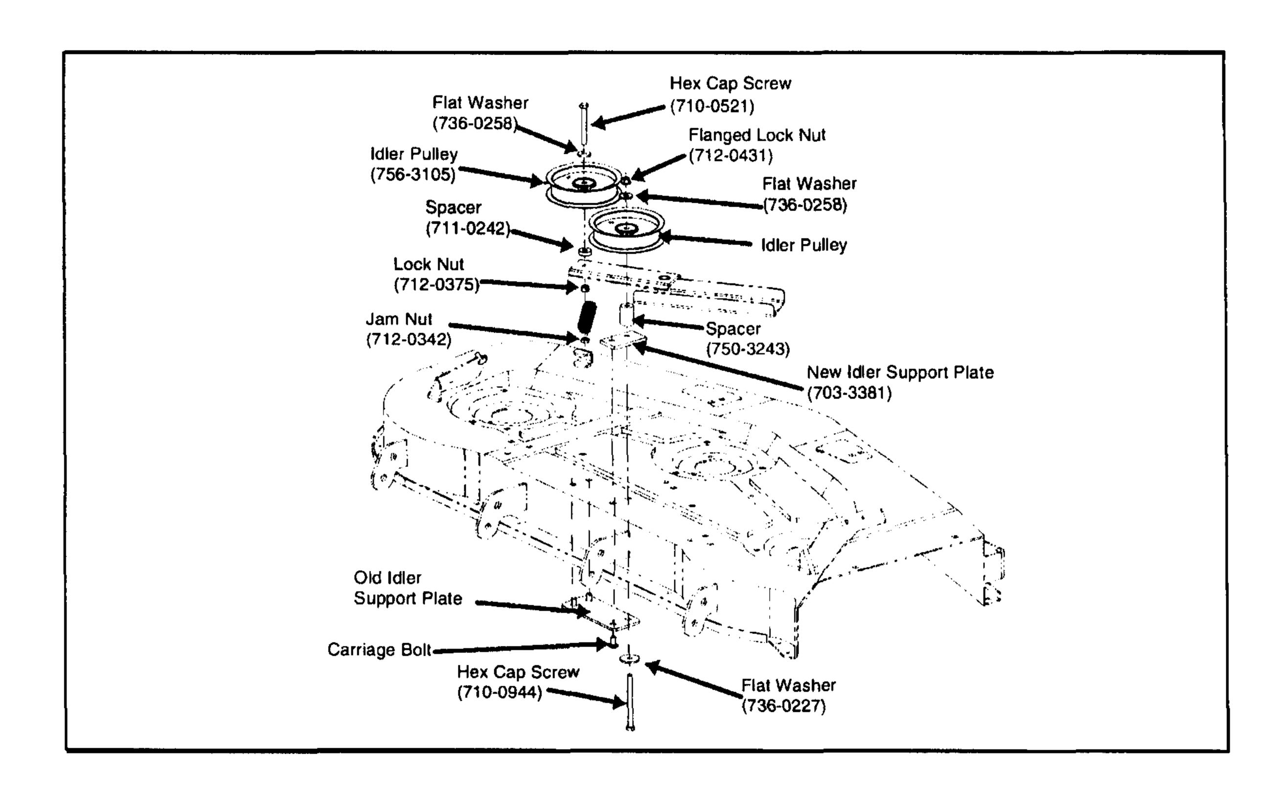
Warranty Allowance: If you get a complaint from a customer of the deck belt jumping off, order and install part number 759-3873 Deck Idler Pulley Kit. The kit will be available from Shelby Parts Distribution at NO CHARGE. Submit a warranty claim in the usual manner for .6 of an hour labor and memo part number 759-3873 at no charge. NOTE: Installation of the no charge kit and labor will be allowed for any unit in dealer's inventory.
