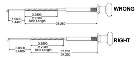
If the cable is wrong, remove/discard the wrong choke cable and replace with part number 746-1085A.
