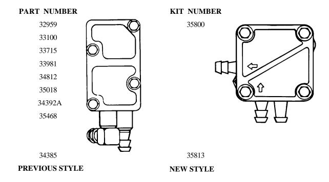
The Pulse Fuel Pump Assembly Kit Part No. 35800 (Kit Part No. 35813 for Part No. 34385 Fuel Pump) supplies all the parts needed to convert the engine from the previous style fuel pump to the new style pump. An instruction sheet explaining the proper installation will be included in each kit.
