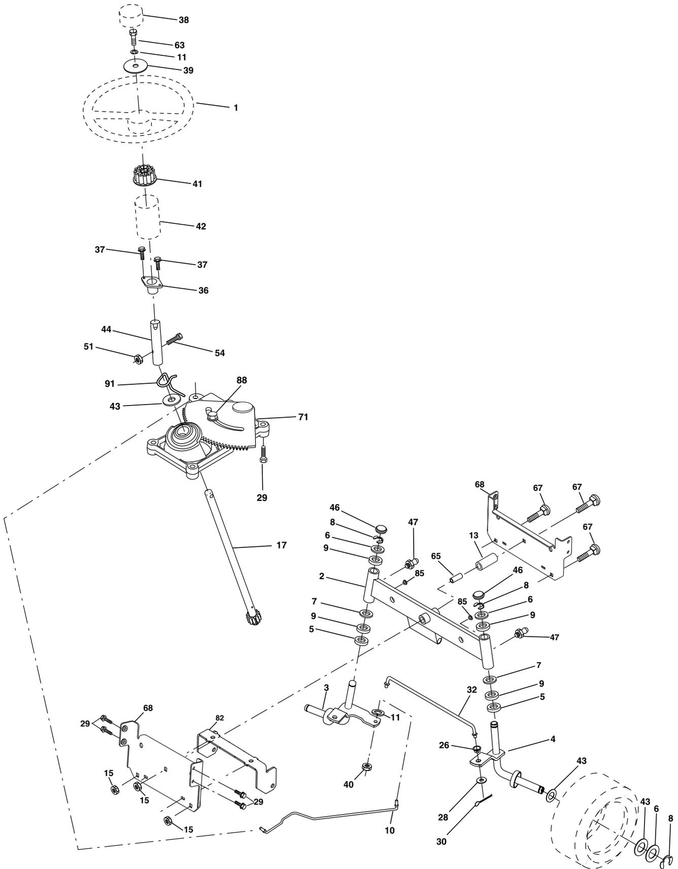
**PIÈCES DE RECHANGE****TRACTEUR - - NUMÉRO DE MODÈLE WE1538A****ENSEMBLE DE LA DIRECTION**
