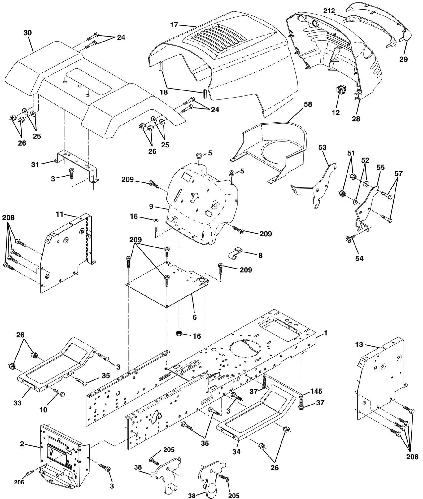
**PIÈCES DE RECHANGE****TRACTEUR - - NUMÉRO DE MODÈLE WE12538J****CHÂSSIS/ENCEINTES**
