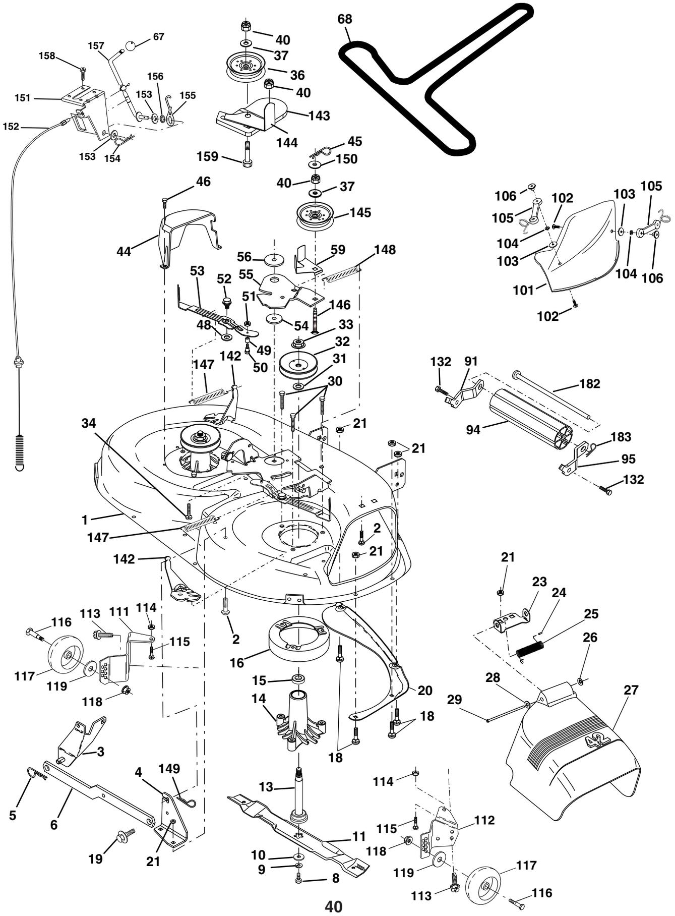
**PIÈCES DE RECHANGE****TRACTEUR-NO. DE MODÈLE PR1842STA NO.DE PRODUIT 954 56 82-05
