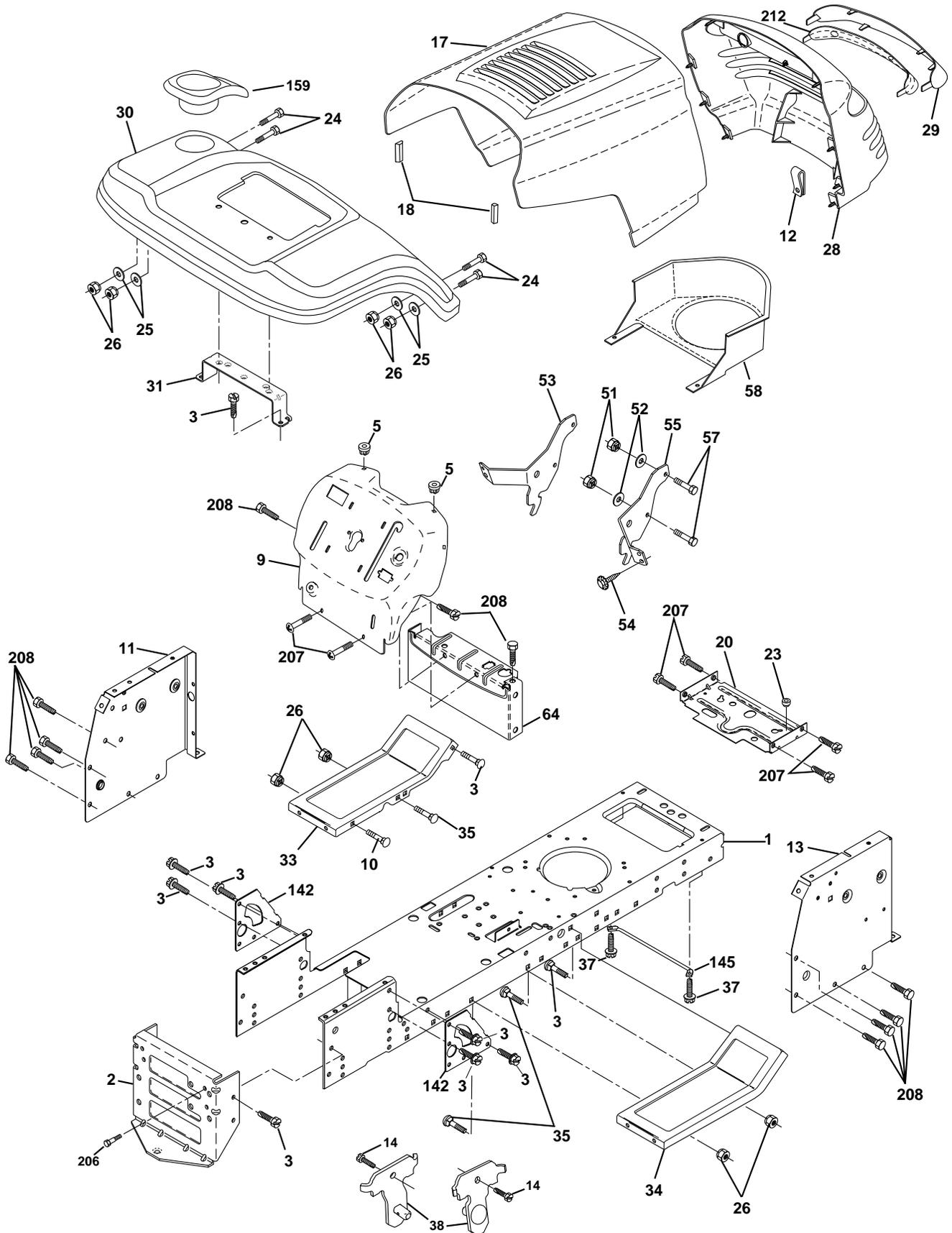
**PIÈCES DE RECHANGE****TRACTEUR-NO. DE MODÈLE PR1742STC****CHÂSSIS ET LES ENCEINTES**
