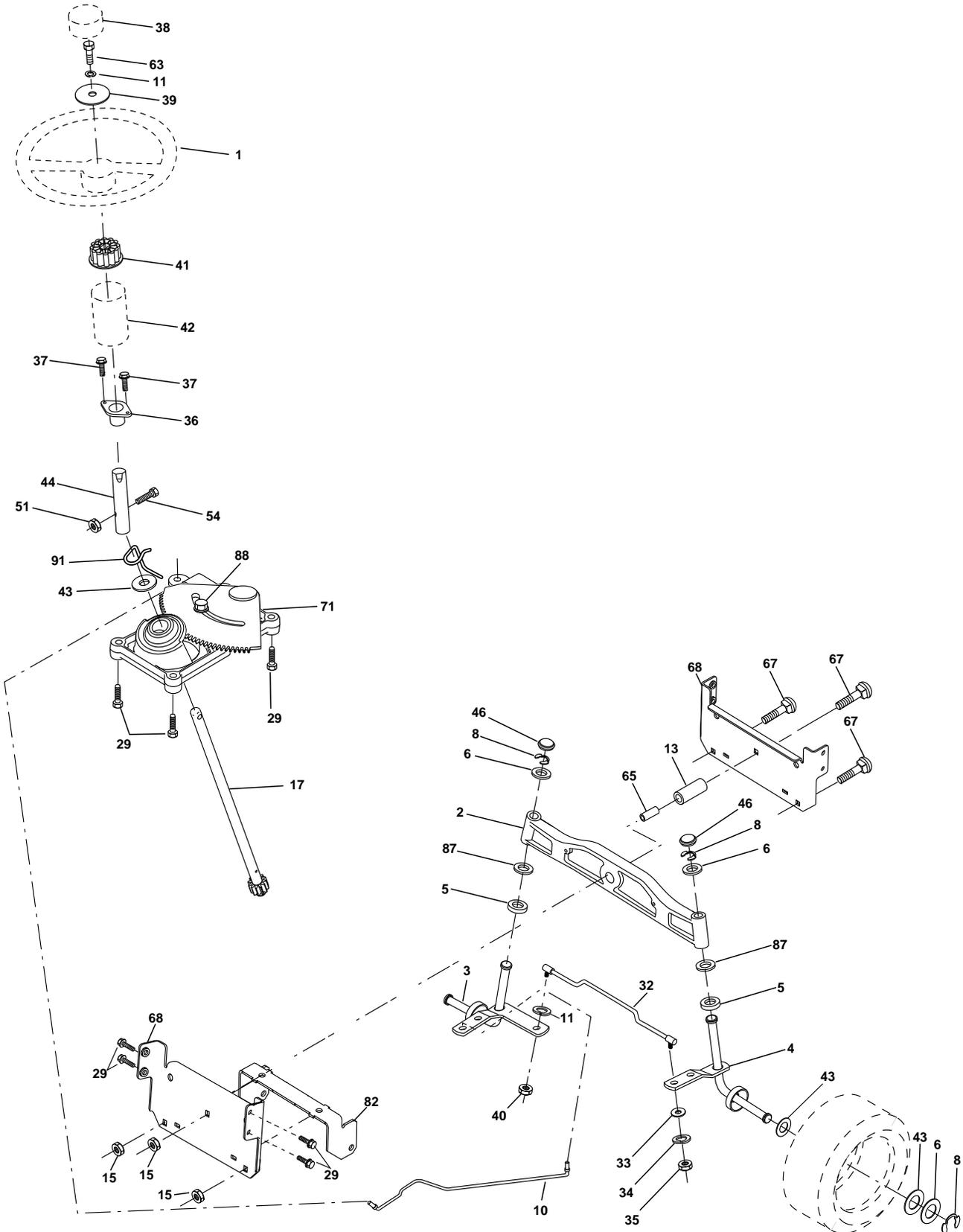
**PIÈCES DE RECHANGE****TRACTEUR-NO. DE MODÈLE PR1742STC****ENSEMBLE DE LA DIRECTION**
