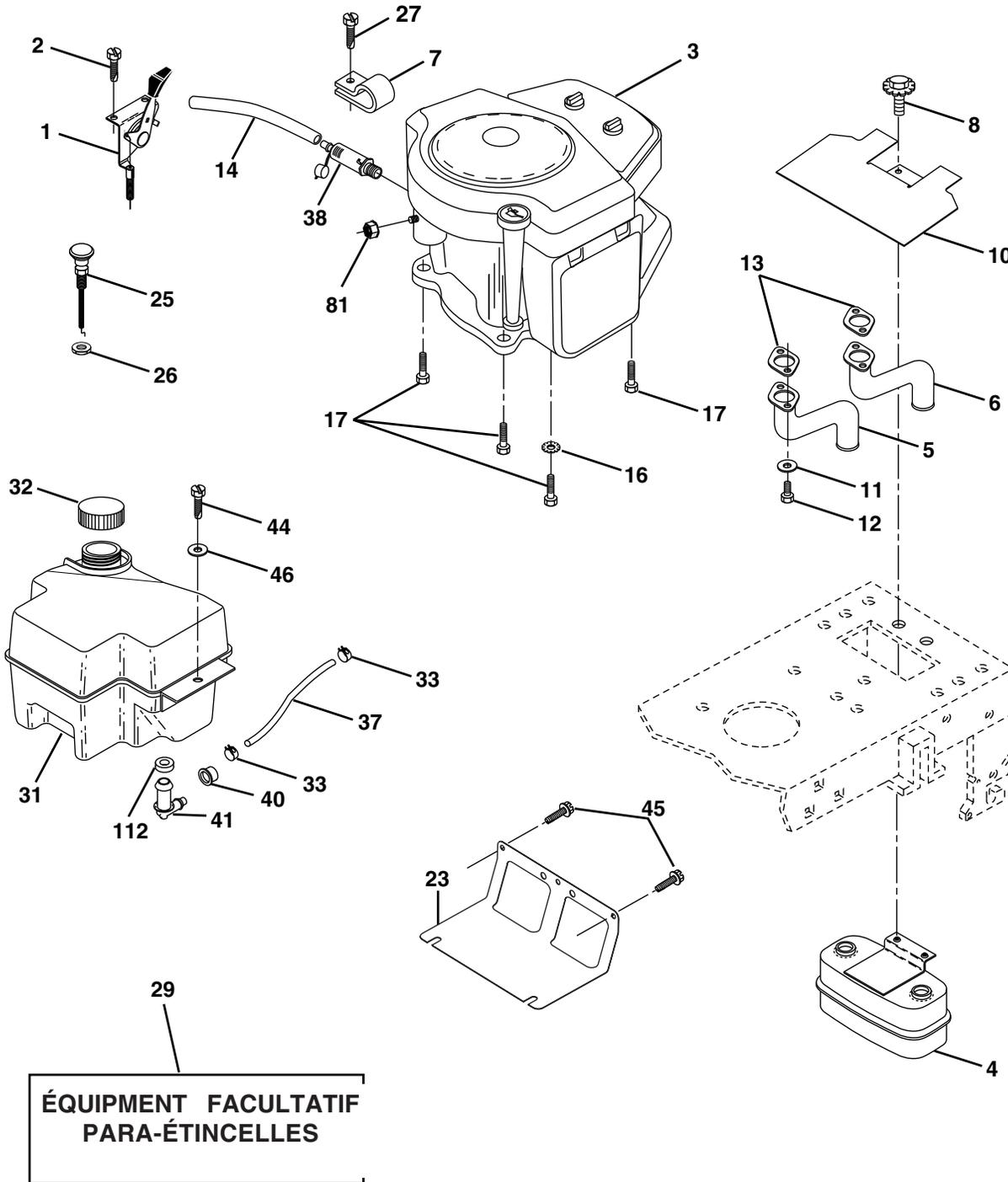
**PIÈCES DE RECHANGE****TRACTEUR - NO. DE MODÈLE PR2042 (PPR2042STB), NO. DE PRODUIT 954 56 84-41
