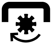
ATTACHMENT CLUTCH ENGAGED
