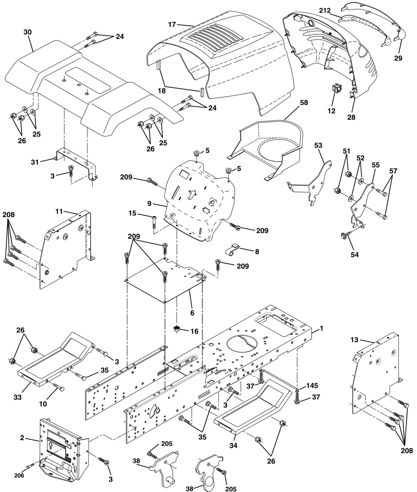
**PIÈCES DE RECHANGE****TRACTEUR - - NUMÉRO DE MODÈLE PO14542D****CHÂSSIS/ENCEINTES**
