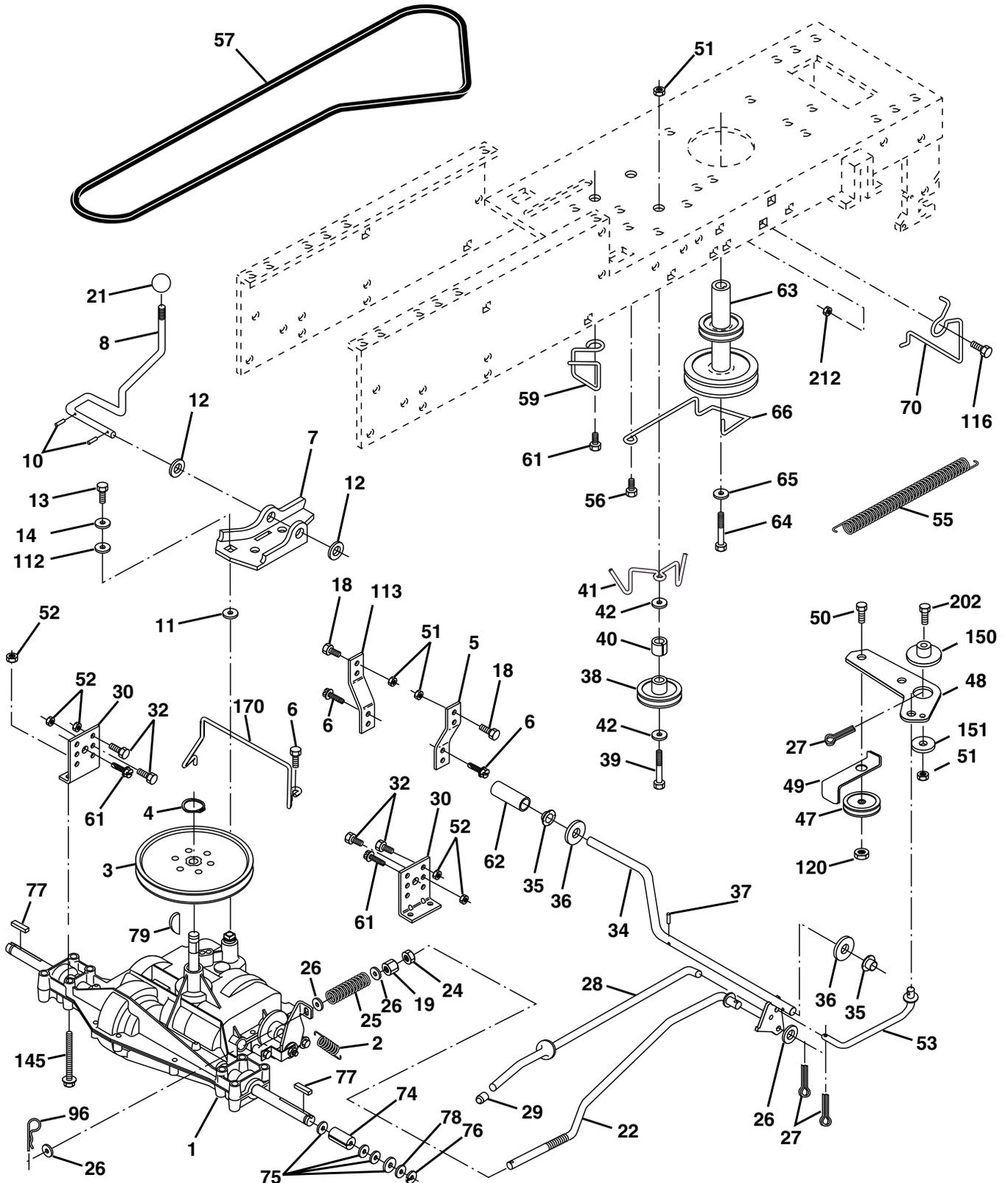
**PIÈCES DE RECHANGE****TRACTEUR - - NUMÉRO DE MODÈLE PO14542D****ENTRAÎNEMENT**
