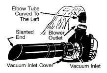
When converting back to the blower feature, make sure that the latch on the vacuum inlet cover is securely fastened.
