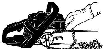
Place chain onto the sprocket
