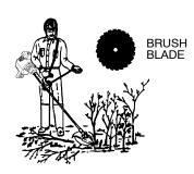
**NOTE:** If your unit has been assembled for trimmer head use, refer to the section ATTACH-ING THE PLASTIC SHIELD AND TRIMMER HEAD and reverse the steps to remove the plastic shield and trimmer head before you mount the metal shield and blade. Store these parts for future use. Never use the trimmer head with the metal blade installed.
