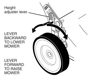
MODELS WITH "QUICK ADJUST" WHEEL HEIGHT ADJUSTERS **NOTE**: For shipping purposes, the rear wheels on your lawn mower may not be adjusted to the same position as the front wheels. Before operating mower adjust all wheels to the same cutting height.
