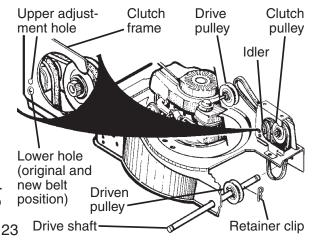
• When reinstalling the belt cover be sure the front hook is under clutch frame. Reinstall in rear of cover.
