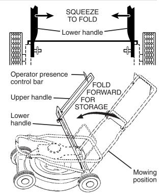
2 POSITION / "ADJUSTABLE" HANDLES When setting you handles up from the storage position, the lower handle will automatically lock into mowing position.
