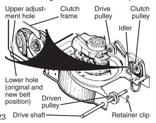
When reinstalling the belt cover be sure the front hook is under clutch frame.
