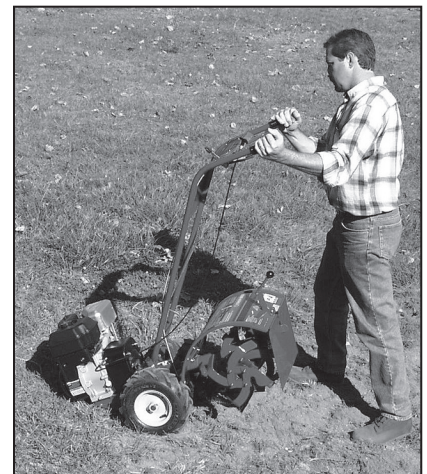
Figure 4-4: To begin turn, reduce engine speed and lift handlebars until engine and tines are balanced over wheels.
