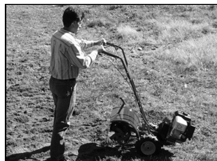
Fig. 4-4: To begin turn, lift handlebars until tines are out of ground and unit is balanced.
