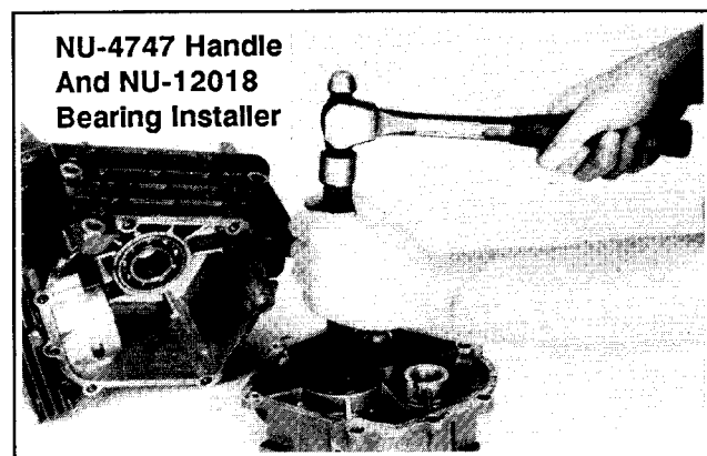
Figure 11-1. Installing Crankshaft Bearings.
