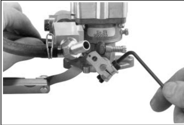
**Figure 5A-10. Tightening Idle Speed Clamp Mounting Screw.**
