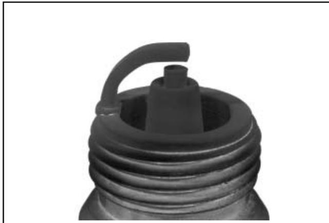
**Carbon Fouled:** Soft, sooty, black deposits indicate incomplete combustion caused by a restricted air cleaner, over rich carburetion, weak ignition, or poor compression.
