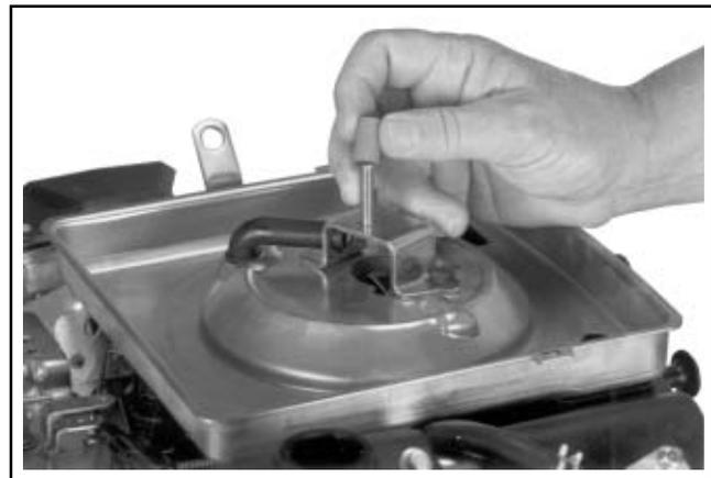
Figure 4-7. Removing Rubber Seal from Bracket.
