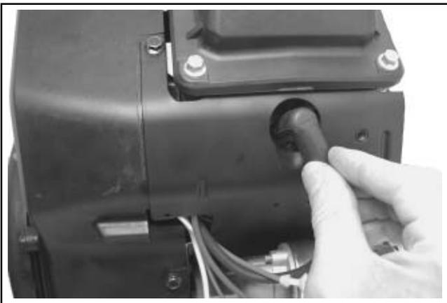
**Figure 11-98. Connect Spark Plug Leads.**
