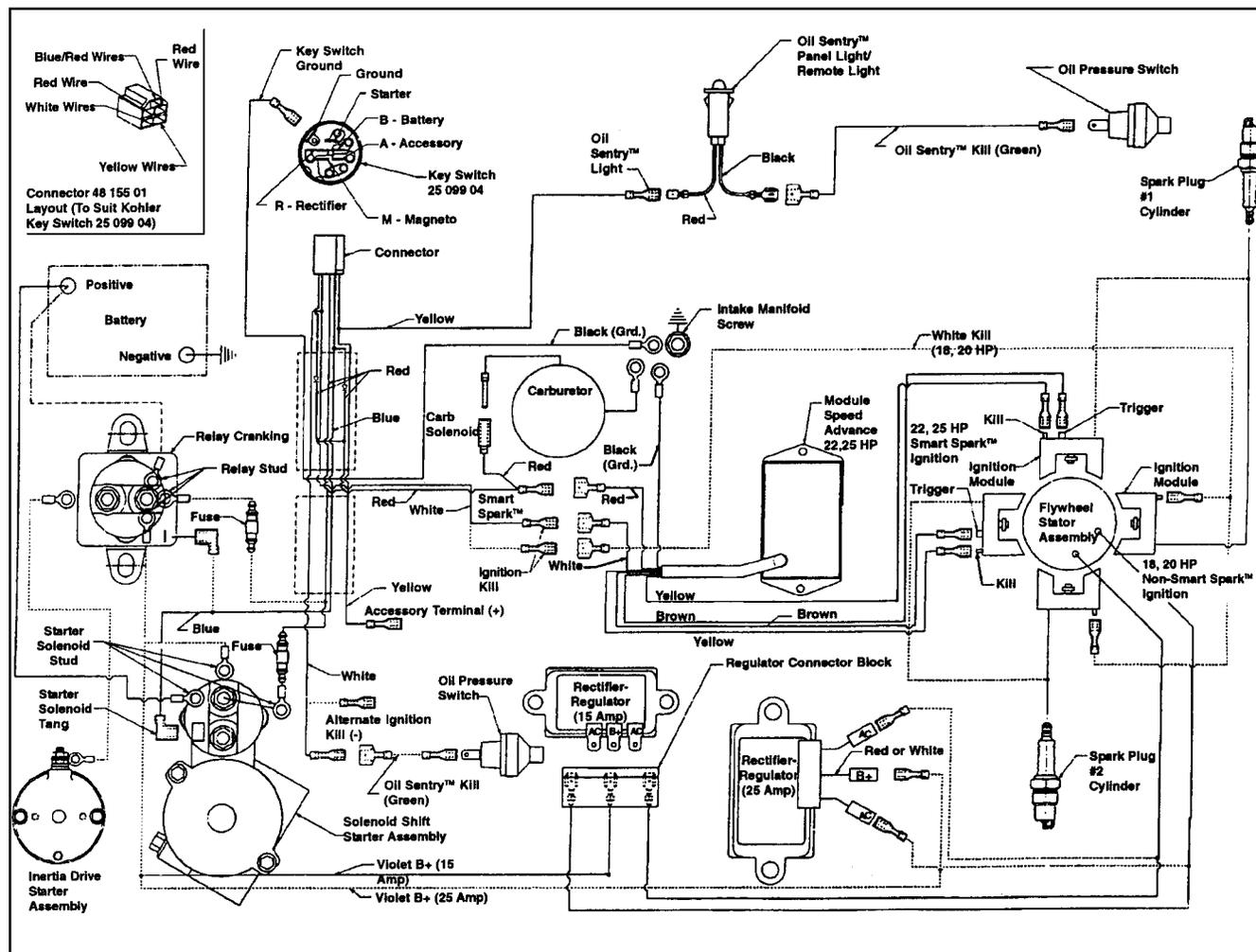
Figure 8-14. Wiring Diagram - 15/20/25 amp Regulated Battery Charging System.
