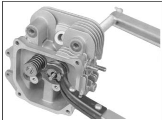
Figure 11-39. Installing Valves with Valve Spring Compressor.
