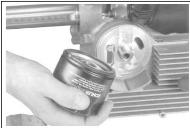
Figure 11-93. Installing New Oil Filter.
