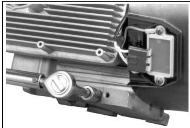
Figure 11-95. Reinstall and Torque Both Oil Drain Plugs.
