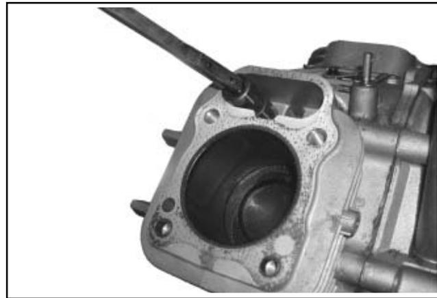
**Figure 9-48. Removing Hydraulic Lifter.**
