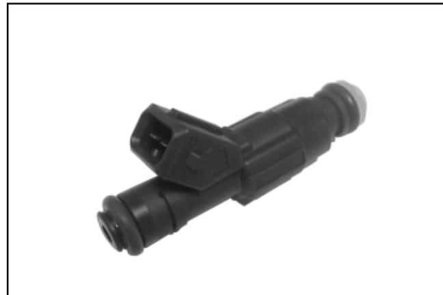
Figure 5B-17. Style 2 Fuel Injector.
