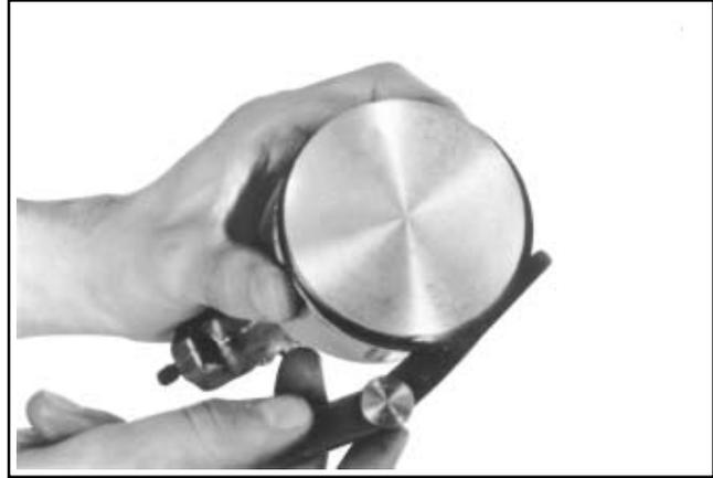
Figure 10-10. Measuring Piston Ring Side Clearance.
