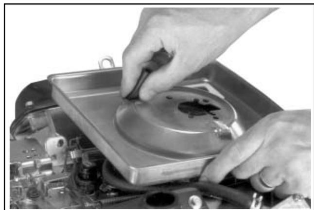
**Figure 9-10. Removing Breather Tube from Base.**
