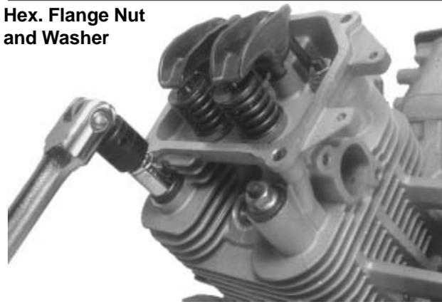
Figure 9-46. Removing Cylinder Head Fasteners.
