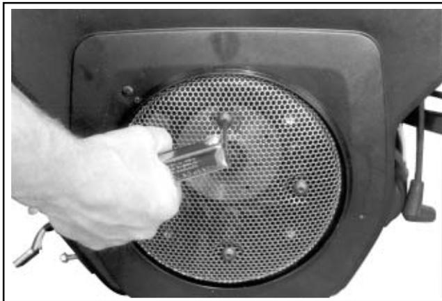
**Figure 9-32. Removing Metal Grass Screen.**
