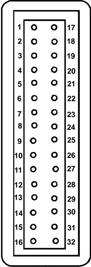
The diagram shows a 32-pin connector with two rows of 16 pins each. The pins are numbered 1 through 32, with the left column numbered 1-16 and the right column numbered 17-32. Each pin is represented by a small circle.
