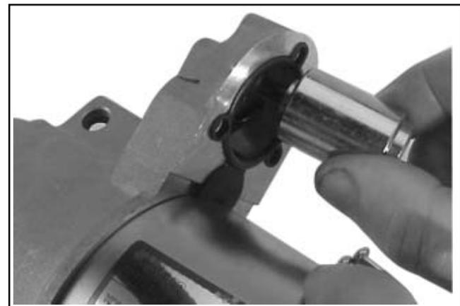
Figure 8-43. Removing Plunger.
