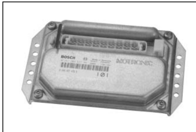
Figure 5B-1. “35 Pin” (MA 1.7) Metal-Cased ECU.
