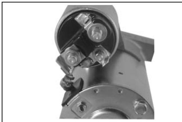
**Figure 8-69. Positive (+) Brush Lead Connection.**
