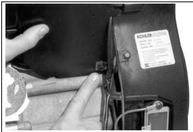
**Figure 9-30. Note Location of Two Short Screws.**
