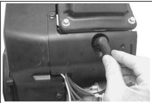
**Figure 11-98. Connect Spark Plug Leads.**
