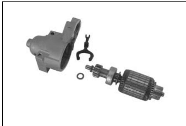
**Figure 8-48. Armature and Lever Removed.**
