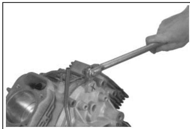
**Figure 9-63. Breaking Seal on Top Splitting Tab.**
