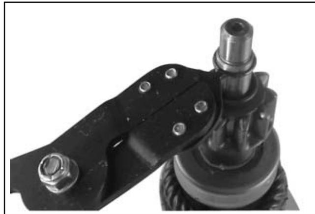
Figure 8-50. Removing Retaining Ring.
