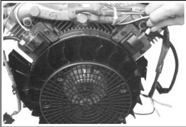
Figure 11-54. Connecting Kill Leads on Standard Ignition Modules.
