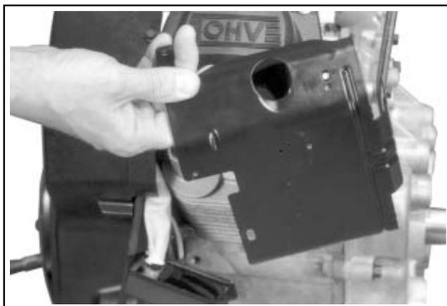
**Figure 9-31. Removing Outer Baffles.**
