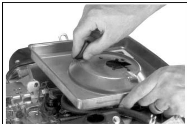
**Figure 9-10. Removing Breather Tube from Base.**
