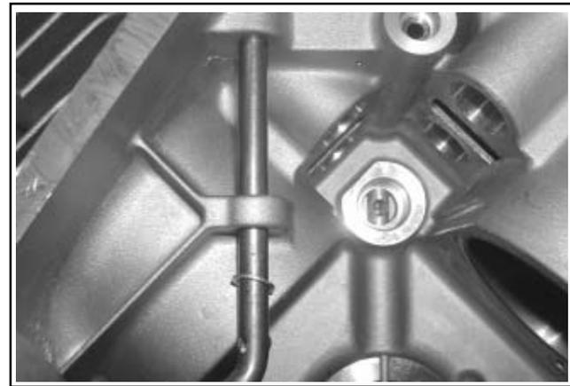
Figure 11-5. Installing 8 mm Governor Cross Shaft.
