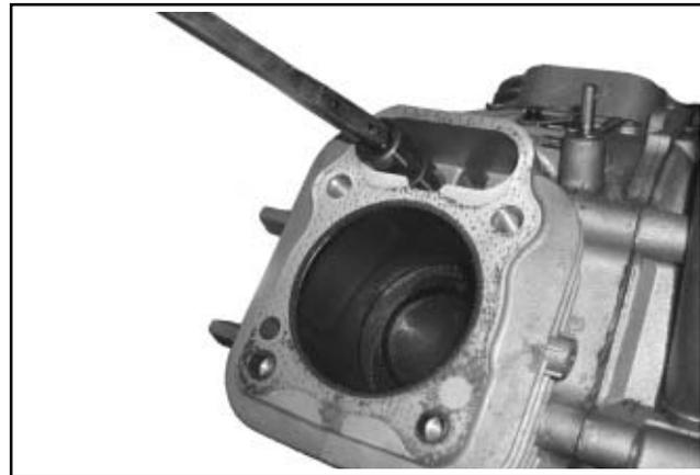
**Figure 9-48. Removing Hydraulic Lifter.**
