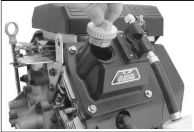
Figure 6-5. Removing Oil Fill Cap.
