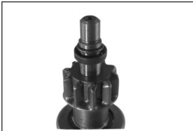
Figure 8-49. Retaining Ring Detail.
