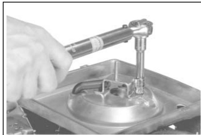
Figure 11-90. Torquing Base Screws.
