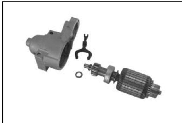
**Figure 8-48. Armature and Lever Removed.**
