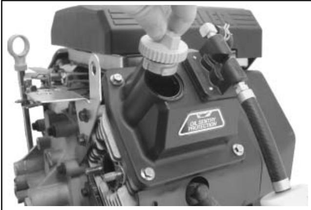
Figure 6-5. Removing Oil Fill Cap.
