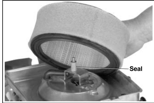
Figure 4-6. Removing Elements.
