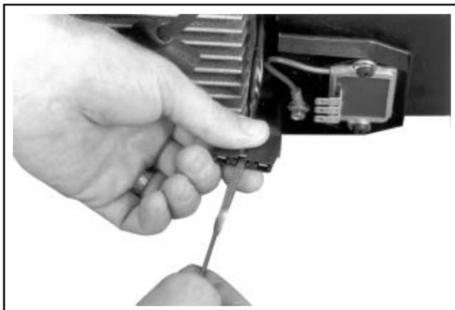
**Figure 9-28. Remove B+ Lead from Terminal Plug.**
