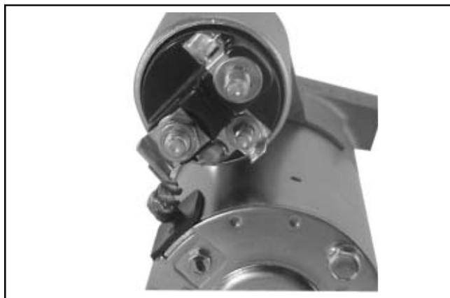
**Figure 8-69. Positive (+) Brush Lead Connection.**
