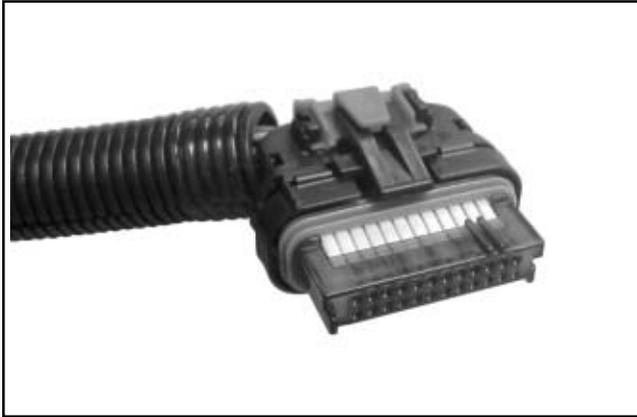
Figure 5B-24. "24 Pin" (MSE 1.0) Plastic-Cased ECU Connector.
