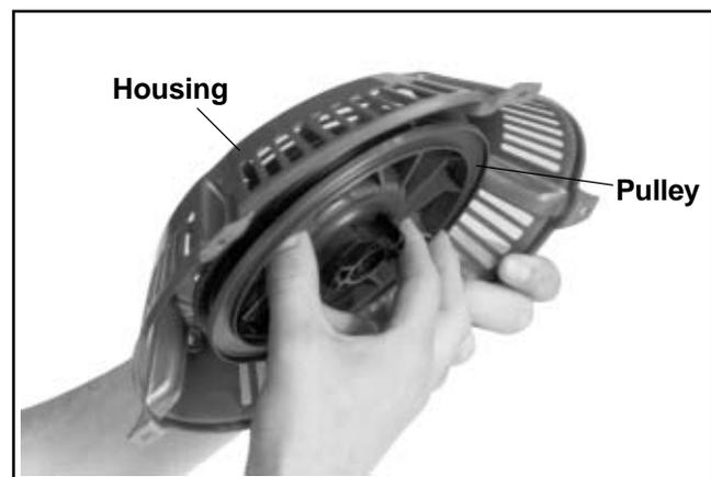
Figure 7-6. Removing Pulley from Housing.
