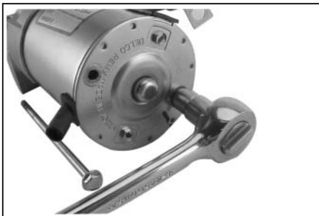
**Figure 8-44. Removing Thru Bolts.**
