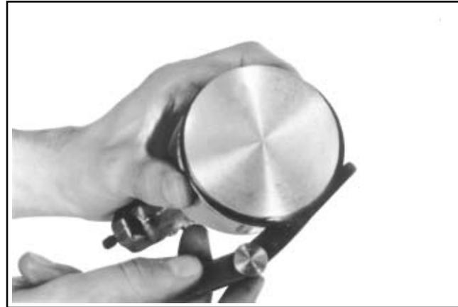
Figure 10-10. Measuring Piston Ring Side Clearance.
