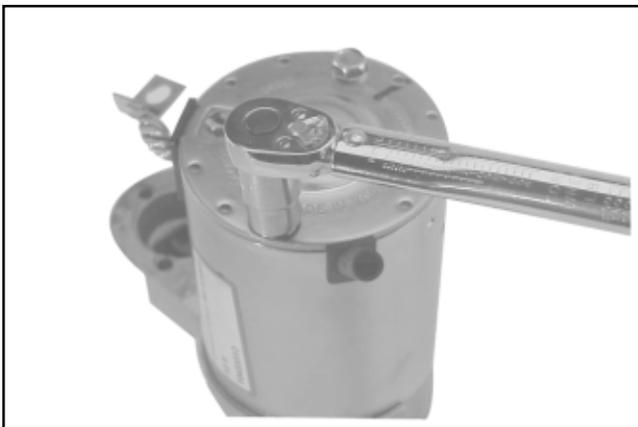
**Figure 8-67. Torquing Thru Bolts.**
