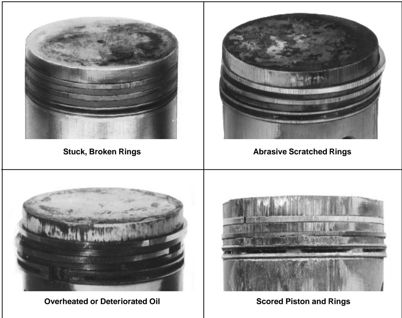
**Figure 10-8. Common Types of Piston Damage.**
