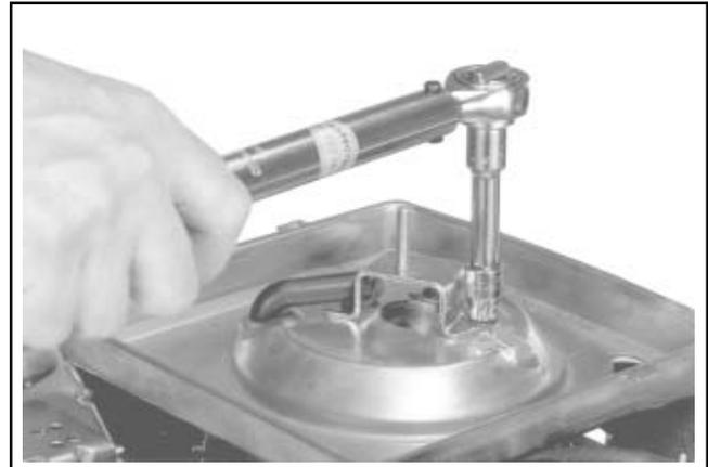
Figure 11-90. Torquing Base Screws.
