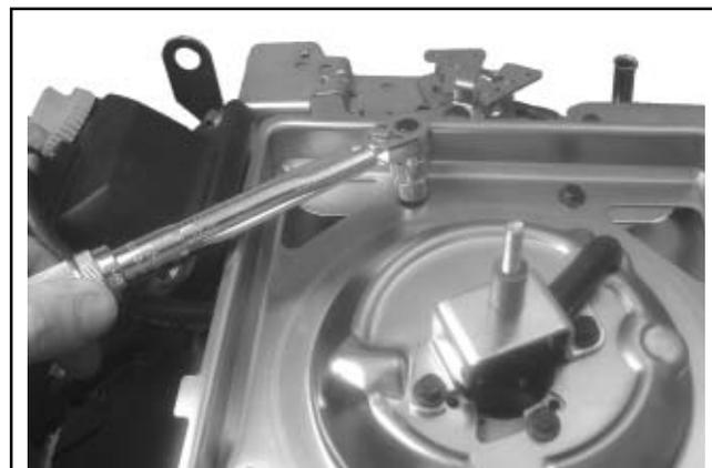
Figure 11-91. Tightening Rear Base/Bracket Screws (Some Models).
