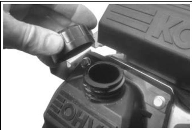
**Figure 11-97. Reinstalling Oil Fill Cap (Some Models).**
