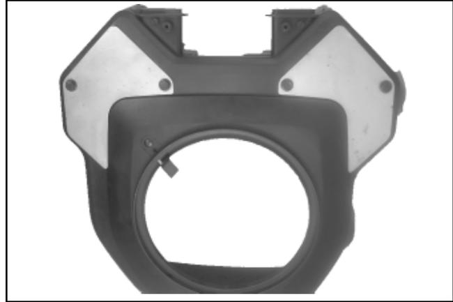
Figure 4-15. Cleanout Kit Installed on Blower Housing.
