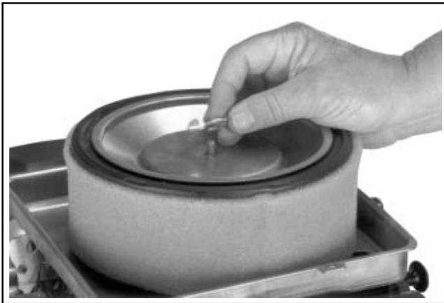
Figure 4-5. Removing Element Cover Wing Nut.
