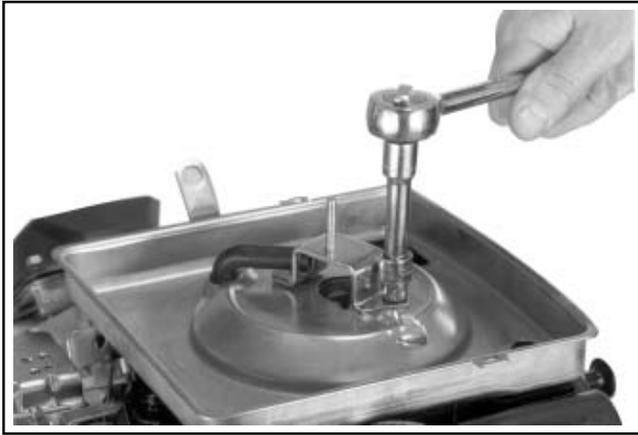
Figure 4-9. Bracket Retaining Screw.
