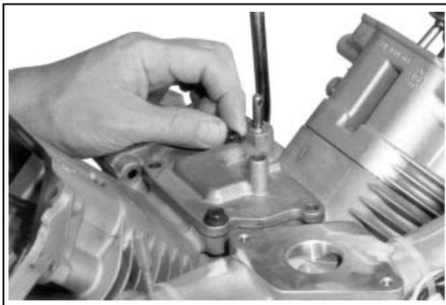
Figure 11-58. Installing Screws (Locations 3 and 4).
