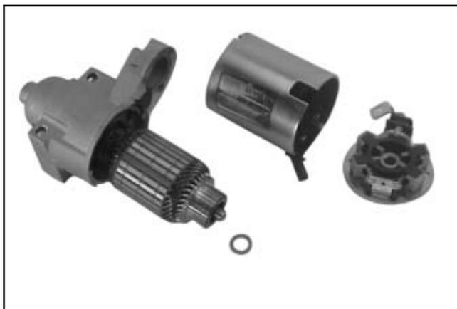
**Figure 8-46. Starter Frame Removed.**
