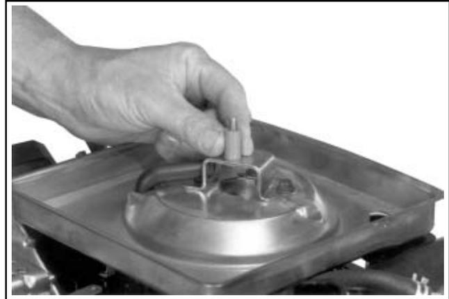
**Figure 9-8. Removing Air Cleaner Base Retainer.**
