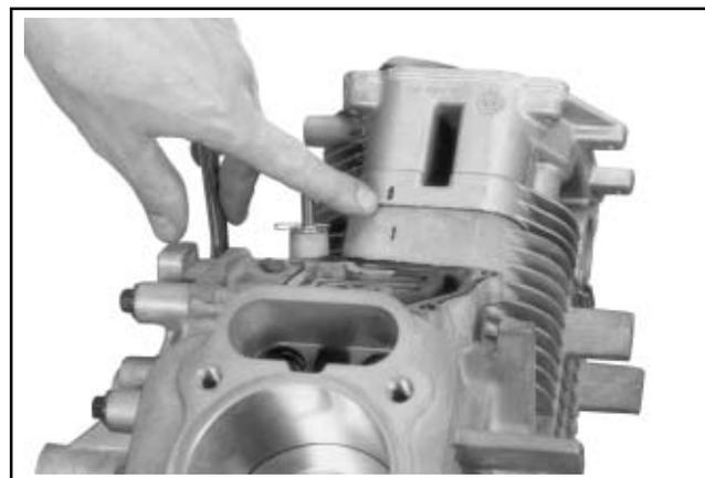
**Figure 9-50. Match Marks on Cylinder Barrel and Heads.**
