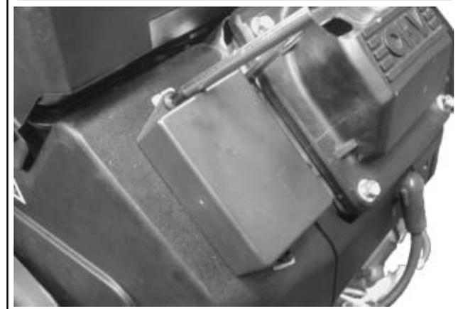
**Figure 9-29. Removing the Spark Advance Module (Applicable Models).**
