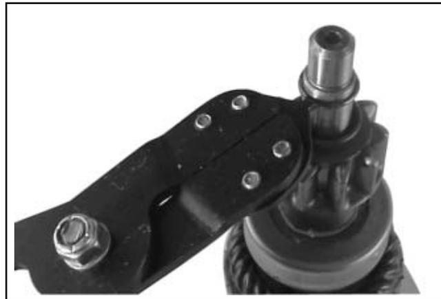
Figure 8-50. Removing Retaining Ring.
