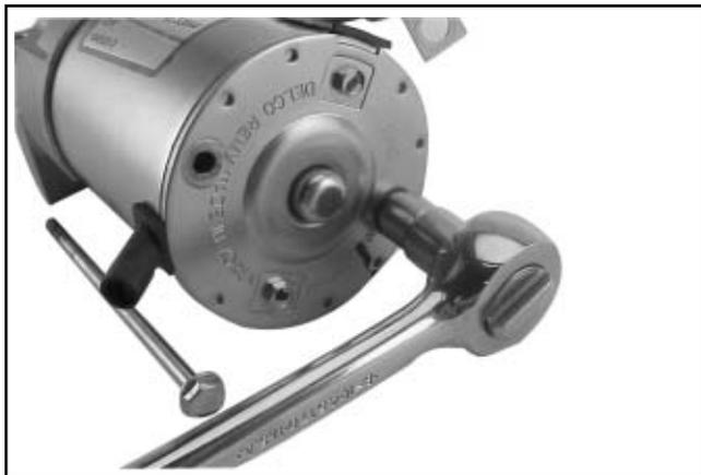
**Figure 8-44. Removing Thru Bolts.**
