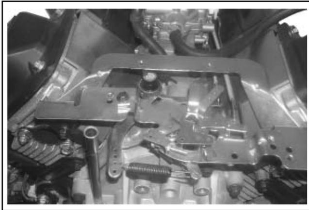
Figure 9-19. Rear Air Cleaner Bracket (Some Models).
