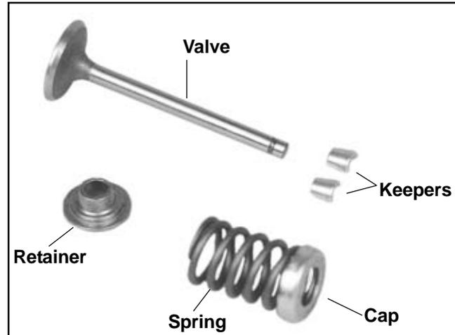
Figure 11-38. Valve Components.
