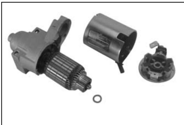
**Figure 8-46. Starter Frame Removed.**
