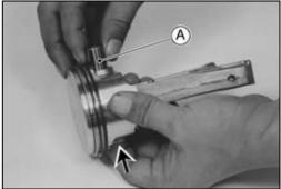
• Remove the piston by pushing the piston pin [A] to the direction from which the snap ring was removed.
