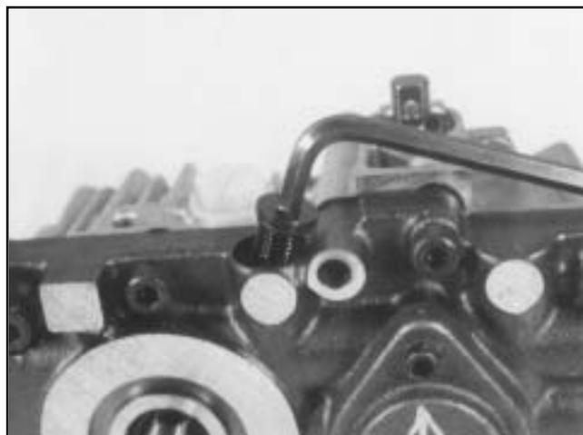
Check Valve Removal/Installation
