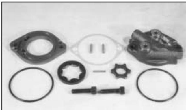
**BDU-21L/A CW Charge Pump Components**
