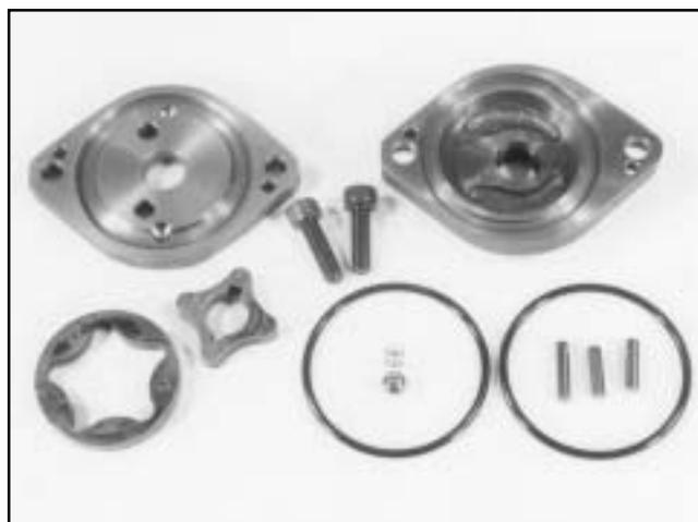
BDU-10L Through Shaft Charge Pump Components
