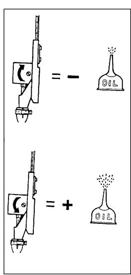
The amount of oil used to lubricate the chain can be adjusted. The standard amount of adjustment is a half turn. Turn screw clockwise to reduce the oil supply and counterclockwise to increase the oil supply.
