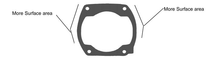
In some case you can still use the old gasket along with a thin coat of gas and oil impervious RTV silicone to insure that it seals. The previous gasket is pictured below.
