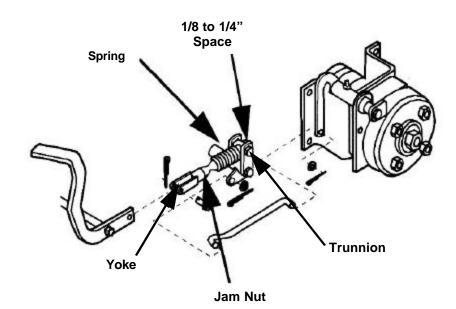
**NOTE:** This brake system has been designed as a parking brake and is intended to hold the unit in place when it is not being operated. It must not be used as an emergency stopping brake, or brake and linkage damage may occur.
