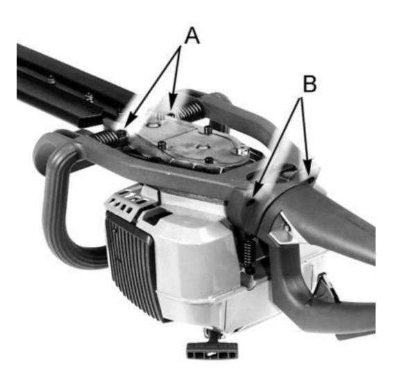
**1**. Disassemble screws "A" and "B". Lift off the front handle.
