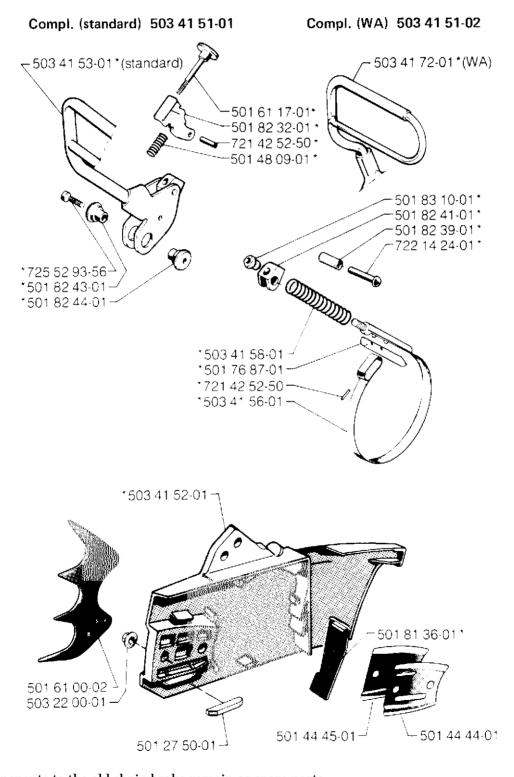
Components to the old chain brake remain as spare parts.
