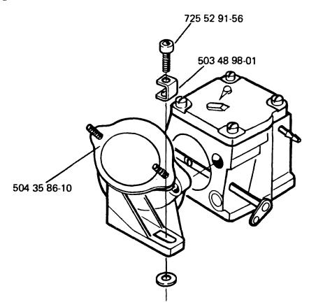
In order to assemble the new carburettor support (the Ref. No. 504 35 86-10 remains) on saws with lower serial number than the above, the following is required:
