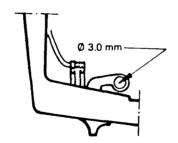
The new stop switch can be mounted on older saws if the terminals on the leads are changed and a hole  $\emptyset$  3.0 mm is drilled in the crankcase. Use the switch as a template. For mounting of new switch there is a rebuilding kit available, which contains:
