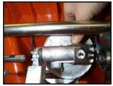
F. Set the shaft, the flat washers and the plastic glide bearing from the top of the variator assembly to the side to be reused. The rubber drive disk and the variator assembly can be discarded.
