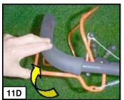
E. If the unit passes these tests, the variator rework is nearly complete. Secure the cable to the handle and ensure it doesn't get caught behind the height adjustment lever when the handle is opened out. Don't forget to reattach the spark plug lead and the grass catcher (or mulch plug if equipped).
