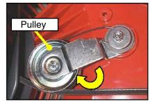
C. Refit the belt cover with the two M6x60 screws (engine side) and two M4x42 screws (discharge side). (Review Step 1 for screw locations.)
