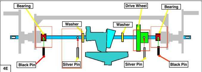
E. The drive shaft is now free to be removed. Carefully, pull the shaft out from one side of the deck while removing the washers, the variator and the rubber drive disk.
