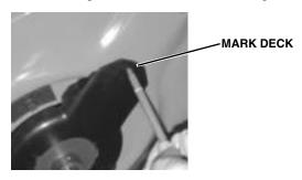
Remove debris shield and drill at the mark a 9/32" (.281) dia. hole in deck.
