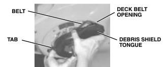
7. Mark deck through hole in debris shield tongue.
