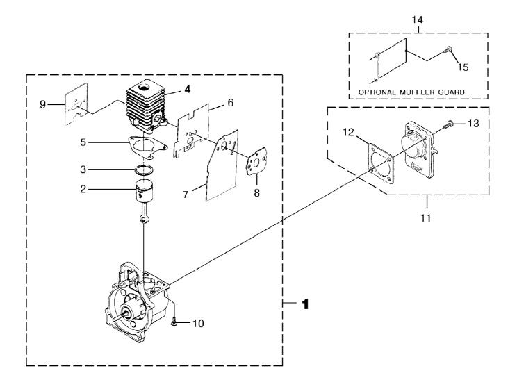
TrimLite String Trimmer UT-20804 Engine Internal
