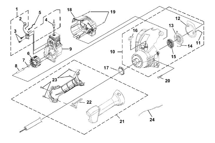
TrimLite String Trimmer UT-20804 Ignition - Rotor - Starter
