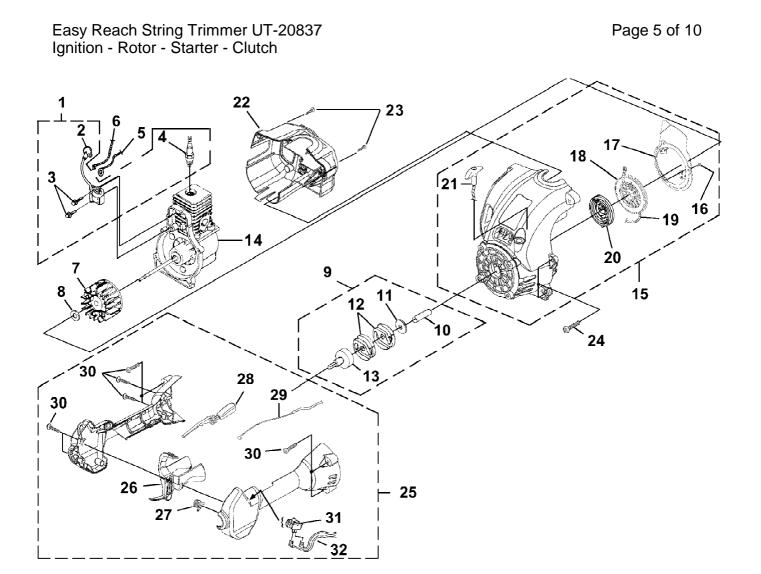
Easy Reach String Trimmer UT-20837 Ignition - Rotor - Starter - Clutch
