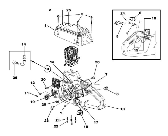
z3800c Chain Saw UT-10785 Engine Housing - Fuel Tank - Oil Tank Page 8 of 14
