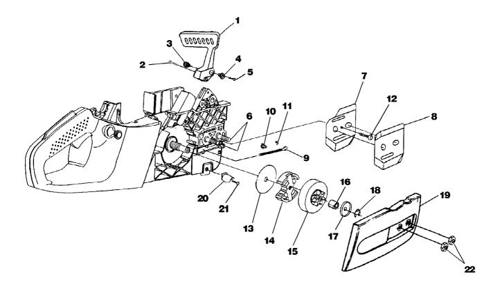
z3800c Chain Saw UT-10785 Clutch - Hand Guard - Drive Case Cover Page 6 of 14
