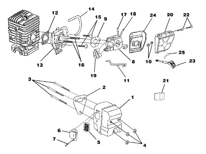
z3800c Chain Saw UT-10785 Carburetor - Muffler - Air Filter Page 4 of 14
