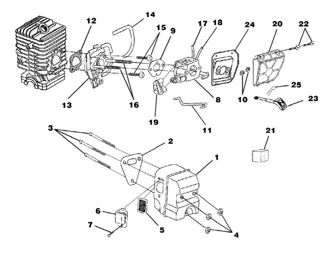
z3300 Chain Saw UT-10782 Carburetor - Muffler - Air Filter Page 4 of 14
