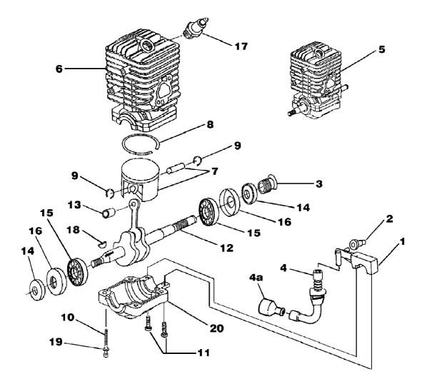
i3350b Chain Saw UT-10774 Engine Internal - Oil Pump Page 10 of 14
