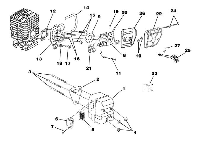
B2718 Chain Saw UT-10877 Carburetor - Muffler - Air Filter Page 4 of 14
