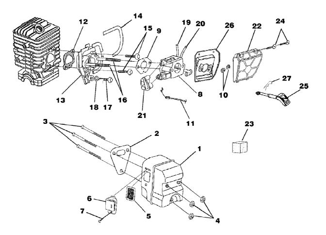
27av Chain Saw UT-10831 Carburetor - Muffler - Air Filter Page 4 of 14
