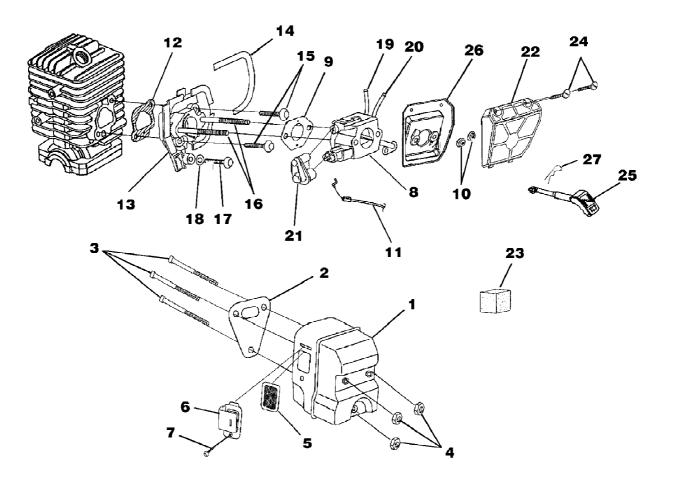
27av Chain Saw UT-10805 Carburetor - Muffler - Air Filter Page 4 of 14
