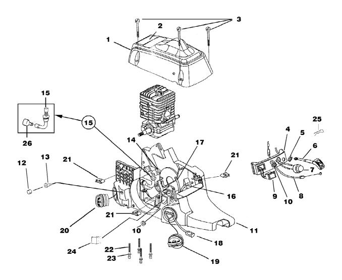
27av Chain Saw UT-10805 Engine Housing - Fuel Tank - Oil Tank Page 8 of 14
