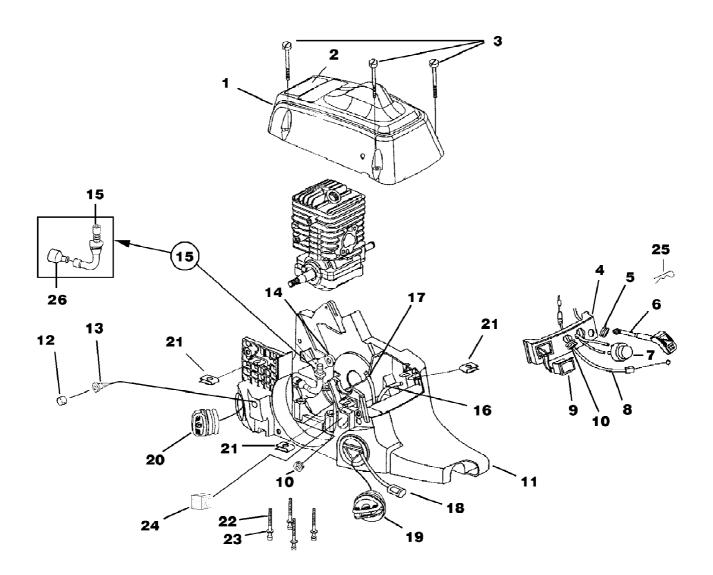
23av w/cc Chain Saw UT-10856 Engine Housing - Fuel Tank - Oil Tank Page 8 of 14
