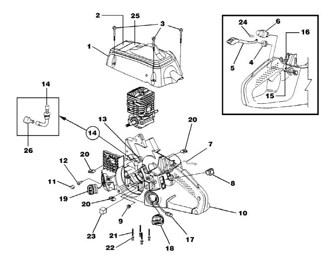
20 w/cc Chain Saw UT-10818 Engine Housing - Fuel Tank - Oil Tank Page 8 of 14
