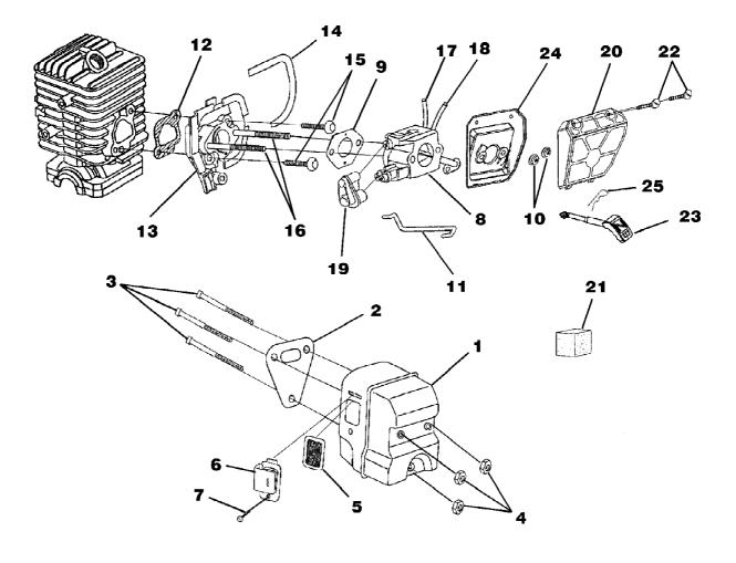
20 w/cc Chain Saw UT-10818 Carburetor - Muffler - Air Filter Page 4 of 14
