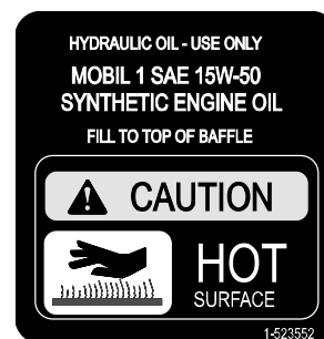
PART NO. 1-523552 LOCATION: Top of Hydraulic Reservoir, Under the Seat
