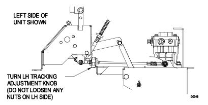
FIGURE 11 LH MOTION CONTROL ADJUSTMENT (S/N 370,000 & HIGHER)
