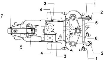
d) Lubricate all control linkages, pivot points, etc., with engine oil or other special lubricant weekly or more often when operating in severe conditions.
