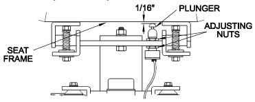
FIG. 11 SEAT SWITCH ADJUSTMENT
