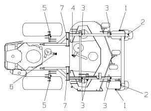
c) Lubricate front caster pivots once a year. Remove hex plug and cap. Thread grease zerk in hole and pump with grease until it oozes out around top bearing. Remove grease zerk and thread plug back in. Place cap back on.
