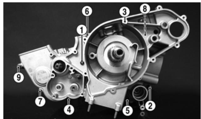
**NOTE:** Cap screw number eight (8) is installed from the right side.
