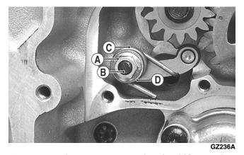
10. Remove the cap screw securing the shift cam plate to the shift cam shaft and remove the shift cam plate; then remove the shift shaft. Account for a washer.
