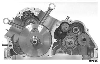
2. Remove the snap ring securing the water pump drive idler (B) to the idler shaft; then remove the drive idler.
