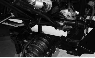
3. Route the brake hose along the lower A-arm shock absorber mount and secure with nylon ties.
