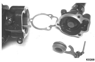
2. Using a T-40 torx wrench, remove the cap screws securing the differential cover. Account for and make note of the ID tag location for assembling purposes.
