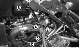
25. Install nylon cable ties at all locations marked prior to removing engine; then check for correct routing of all wiring, hoses, and cables.
