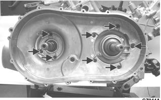
9. Place the driven pulley assembly into position and secure with the nut (coated with red Loctite #271). Tighten to 80 ft-lb.
