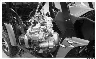
2. Carefully lower the engine/transmission into position between the engine mounting tabs being careful to keep all cables, wires, and hoses clear; then install the longer, front through-bolt with a flat washer.
