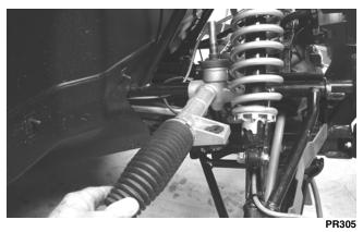
2. With the rack and the steering wheel centered, slide the lower steering shaft joint onto the pinion shaft aligning the match marks.
