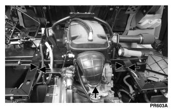
16. Disconnect the engine/harness ground; then disconnect the starter cable from the starter.
