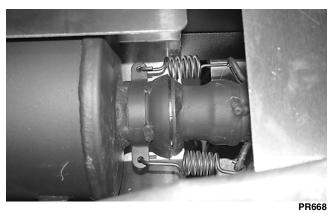
11. Connect the oil cooler hoses to the engine and secure with the hose clamps. Tighten securely.
