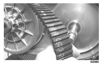
■NOTE: The arrows on the V-belt should point forward.
