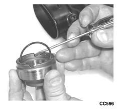
■NOTE: Account for and inspect the clutch housing seal.
