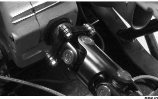
27. Remove the lock nuts from the engine through-bolts; then attach a lifting chain to the engine/transmission.
