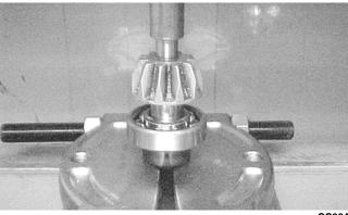
3. Install the pinion gear assembly into the housing. Using the 48 mm Internal Hex Socket, secure the pinion gear assembly with the existing lock collar. Tighten to 120 ft-lb.
