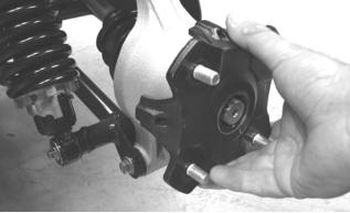
5. Remove the cap screw and lock nut securing the knuckle to the upper A-arm. Discard the lock nut.
