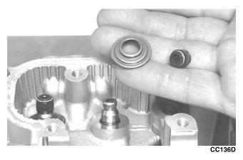
■NOTE: The valve seals must be replaced.
