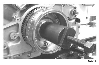
■NOTE: The puller has left-hand threads.
