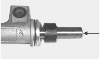
4. Coat the thread with red Loctite #271; then install the tie rod into the rack and using an appropriate crow-foot, tighten to 59 ft-lb.
