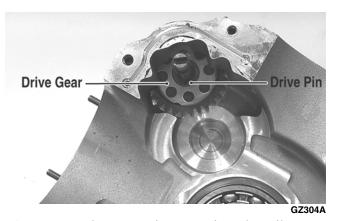
4. Remove the snap ring securing the oil pump driven gear (D) to the oil pump driveshaft; then remove the gear. Account for a drive pin and washer.
