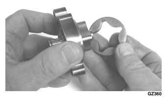
4. Place a new O-ring seal on the outside of the oil pump cover. The oil pump assembly is now ready for assembly into the crankcase.
