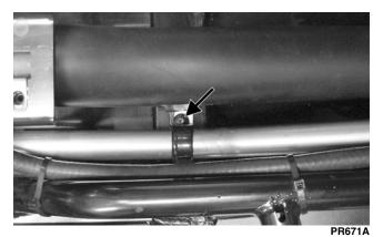
20. Remove the inlet boot from the CVT housing; then remove the outlet boot from the rear of the CVT housing.
