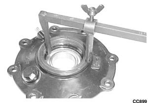
2. Using a press, remove the bearing.
