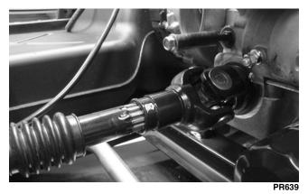
6. Align the match mark on the front drive flange to mark on the front universal joint flange and secure with three cap screws. Tighten to 40 ft-lb and slide the rubber boot back into position.
