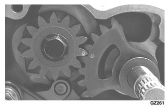
9. Apply grease to the lips of the shift shaft seal in the shifter housing; then using a new gasket, install the shifter housing and secure with the cap screws. Tighten in a crisscross pattern to 8 ft-lb.
