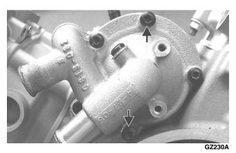
■NOTE: The water pump is a non-serviceable component and must be replaced as a complete assembly.
