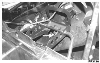
2. Apply green Loctite #270 to the cap screw; then install the cap screw in the upper steering shaft joint. Install the nut and finger-tighten.
