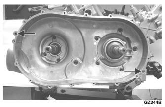
2. Remove the nut securing the movable drive face; then remove the face. Account for a spacer and a flat washer.
