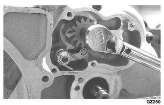
8. Install the shift shaft into the crankcase making sure the washers are properly located; then align the timing reference marks and completely seat the shift shaft.
