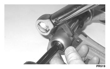
■NOTE: Always attach the crow-foot to the torque wrench with the open end 90° to the torque wrench handle to ensure accurate torque application.
