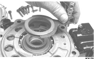
5. Remove the left differential bearing flange assembly and account for a shim. Mark the shim as left-side.
