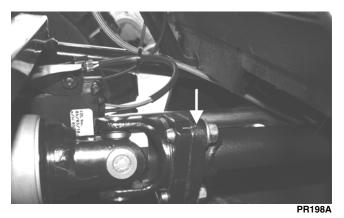
14. Using a slide hammer, remove the front axles.
