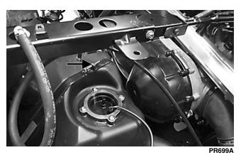
4. Place the gas cap filler panel into position; then if necessary, position the gas tank so the filler panel and filler neck are not binding or rubbing.
