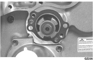
12. Remove the cap screws securing the oil filler cover to the crankcase; then remove the cover. Account for an O-ring.
