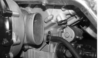
22. Remove two springs securing the muffler to the exhaust pipe and remove the muffler. Account for a grafoil seal.
