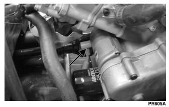
17. Disconnect the crankcase breather hoses from the crankcase and auxiliary drive cover and remove the separator tank and breather hoses.
