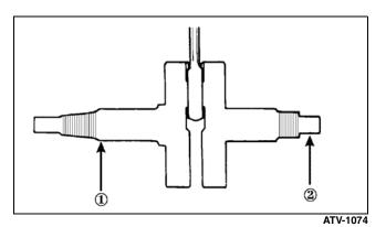
3. Zero the indicator and rotate the crankshaft slowly.
