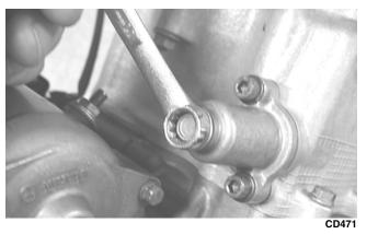
31. Loosen the four adjuster screw jam nuts; then loosen the four adjuster screws on the rocker arms in the valve cover.
