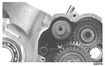
6. Remove two cap screws securing the oil pump in the crankcase and remove the oil pump.
