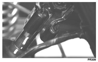
3. Apply green Loctite #270 to the cap screw; then place the lower steering shaft joint to the pinion shaft with the cap screws making sure the shaft does not protrude into the joint beyond the clamping surface.
