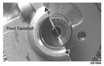
14. Seat the cam sprocket onto the camshaft making sure the alignment pin in the camshaft aligns with the smallest hole in the sprocket; then place the camshaft/sprocket assembly onto the cylinder ensuring the following.
