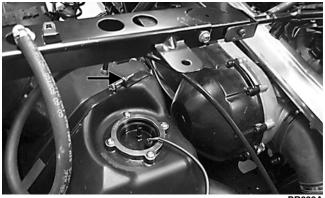
9. Lift and slide the tank forward raising the front of the tank first; then turn the tank and lift out the right side.
