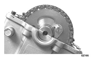
17. Keeping tension on the opposite cam chain, rotate the crankshaft until the second cap screw securing the sprocket to the camshaft can be installed; then install the cap screw (threads coated with red Loctite #271) and tighten to 11 ft-lb. Bend the tab to secure the cap screw.
