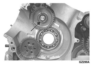
3. Remove the water pump driven shaft (C). Account for the driven gear and drive pin.
