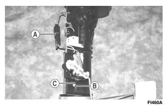
B. Engage the tabs (C) of the fuel level sensor into the mounting slot (B) and press toward the bottom of the fuel pump to latch in place; then connect the two-wire connector (A).
