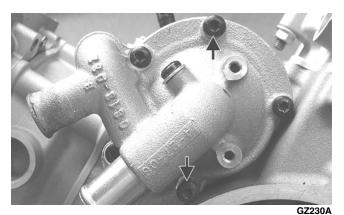
3. Remove the water pump from the engine.
