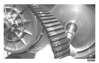
■NOTE: The arrows on the V-belt should point in direction of engine rotation (forward).
