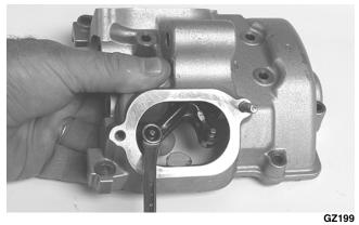
32. Apply a thin coat of Three Bond Sealant to the mating surfaces of the cylinder heads.
