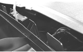
4. Drain the coolant into a suitable container; then disconnect the cooling fan wire connector from the main harness.
