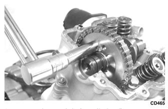
25. Rotate the crankshaft until the first cap screw (from step 23) can be addressed; then tighten to 11 ft-lb. Bend the tab to secure the cap screw.
