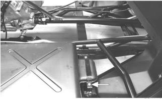
4. Remove the gas tank filler neck shroud; then move the gas tank forward enough to remove the constant variable transmission (CVT) cover. Install the gas cap.
