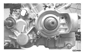
8. Making sure the alignment pins are correctly installed, place a bead of silicone sealant on the mating surfaces and install the V-belt housing. Secure with the cap screws tightened to 8 ft-lb.
