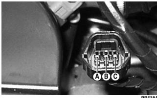
4. Remove the black tester lead from terminal A and connect it to terminal C. The meter should read 5.0 DC volts.
