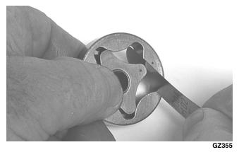
4. Inspect the oil pump cover for scoring, discoloration, or cracks. Replace if damaged.
