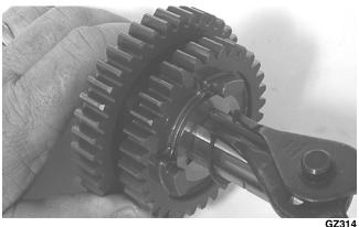
5. Install the reverse driven gear dog onto the countershaft and secure with a snap ring.
