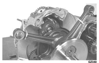
2. Coat both sides with motor oil; then install the spacer washer on the crankshaft with the radius directed toward the crankshaft.
