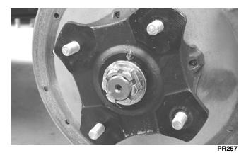
3. Remove the flange nut securing the hub.
