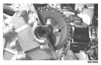
7. While holding the chain, slide the sprocket and camshaft out of the cylinder head.
