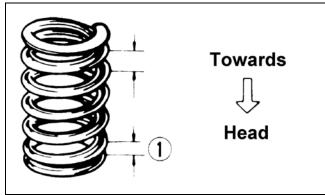
4. Place a spring retainer over the valve springs; then using the valve spring compressor, compress the valve springs and install the valve cotters.
