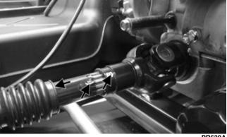
26. Remove four cap screws securing the rear driveshaft to the output flange. The rear driveshaft can remain on the vehicle.
