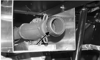
23. Remove two cap screws securing the front exhaust pipe to the cylinder head; then remove two springs securing the front and rear exhaust pipes together. Remove the front exhaust pipe. Account for a grafoil seal and a grafoil gasket.
