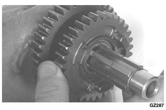
4. Install the outer reverse driven washer; then secure the reverse driven gear assembly with a snap ring.
