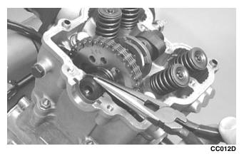
27. Install the cylinder head plugs in the cylinder heads with the open end facing downward and toward the inside.
