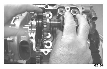
■NOTE: At this point, oil the camshaft bearings, cam lobes, and the three seating journals on the cylinder.
