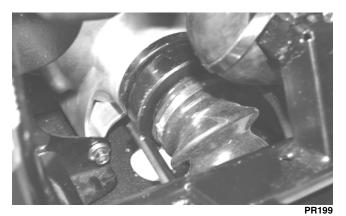
15. Remove the lower differential mounting cap screw. Account for a lock nut and four washers. Note the position of the washers for assembling.
