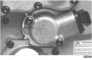
5. If removed, install the shift cam stopper on the support; then with the flat washer in place, install the shift cam stopper assembly into the crankcase and tighten to 8 ft-lb.
