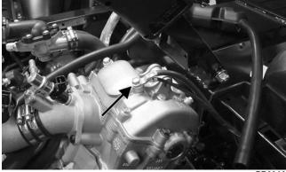
15. Install the air filter assembly and secure with four sheet metal screws; then secure the intake boot to the throttle body. Tighten the screws and clamp securely.
