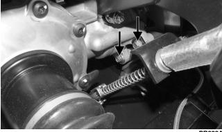
4. Remove the two lock nuts (A) from the brake pad anchor bolts; then remove the brake pads (B). Account for two springs and spacers (C).
