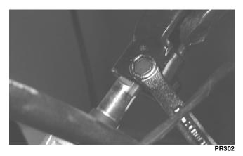
Remove two cap screws securing the rack and pinion assembly to the frame. Account for two nuts and two washers.
