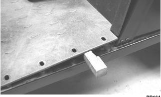
4. From the opposite side of the vehicle repeat step 3; then lift the rear of the floor up and lift the floor out of the vehicle.
