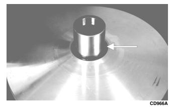
7. Install one of the CVT cover cap screws into the driven pulley fixed face; then turn the cap screw clockwise to spread the pulley faces. Remove the V-belt.
