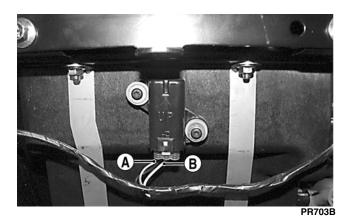
4. Tilt the sensor 60° or more to the left and right observing the meter. The meter should read 4.0-8.0 DC volts after approximately one second in the tilted position. If the meter readings are not as specified, the tilt sensor is defective.
