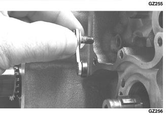
6. Install the shift cam stopper spring onto the shift cam stopper and secure with a flat washer and flange nut. Tighten to 8 ft-lb.
