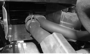
9. Install the two springs at the juncture of front and rear exhaust pipes.
