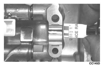
6. If clearance is excessive, measure the journals of the camshaft.
