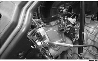
20. Install the shift cable support bracket and secure with two cap screws; then tighten to 8 ft-lb and install the E-clip securing the shift cable to the shift arm.
