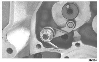
7. Install the shift cam plate onto the shift cam shaft and secure with the cap screw. Tighten to 8 ft-lb.
