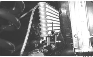
2. Remove the flange nuts and cap screws from the oil cooler mountings and remove the oil cooler.
