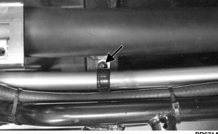
13. Install and secure the CVT cooling outlet boot to the CVT housing making sure to properly orient the outlet duct.
