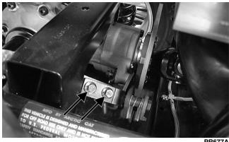
8. Connect the brake cable to the actuator arm with the pin and flat washer and secure with the cotter pin; then adjust the parking brake (see ADJUST-ING in this sub-section).
