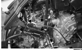
23. Connect the front spark plug cap and front ignition coil; then install the front and rear injector connectors (A), MAP sensor (B), parking brake warning switch (C), reverse override switch connector (D), and ISC valve (E).
