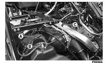
6. Remove the outer cap screw securing the front tank hold-down; then swing the hold-down to the left.
