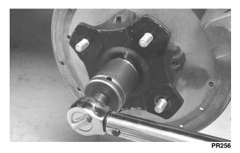
Install a new cotter pin and secure by spreading as shown.
