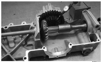
3. While rocking the drive bevel gear back and forth, note the maximum backlash reading on the gauge.
