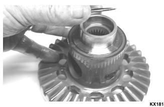
7. Using the 48 mm Internal Hex Socket, remove the lock collar securing the pinion gear assembly.
