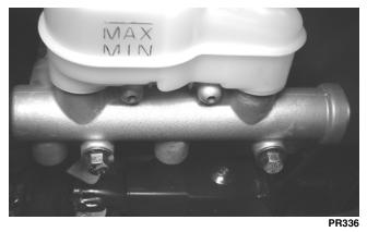
3. Remove the oil bolt securing the banjo-fittings to the master cylinder; then remove the master cylinder. Discard the three crush washers.
