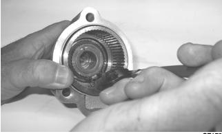
5. Using a new gasket, install the assembled rear drive input shaft/housing onto the rear drive gear case and secure with the three cap screws. Tighten to 23 ft-lb.
