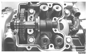
33. Lubricate the camshaft journals and lobes with engine oil; then place the valve cover into position.
