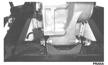
16. Remove the upper differential mounting cap screw. Account for a lock nut and two washers.
