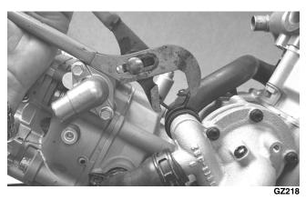
7. Remove the two cap screws securing the water pump to the crankcase; then remove the water pump. Account for an O-ring.
