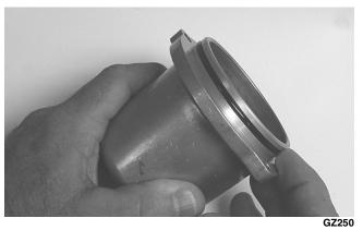
3. Clean the countershaft and trigger splines thoroughly and install the inner snap ring onto the shat; then apply green Loctite #620 to the trigger and countershaft splines and install the trigger. Secure with a flat washer and outer snap ring.
