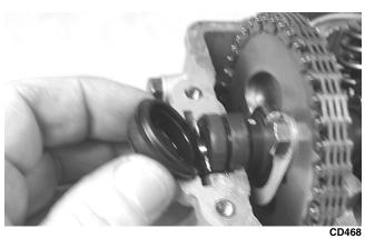
28. Remove the cap screw from the end of the chain tensioner; then using a flat-blade screwdriver, rotate the adjuster screw inside the tensioner clockwise until the screw bottoms.
