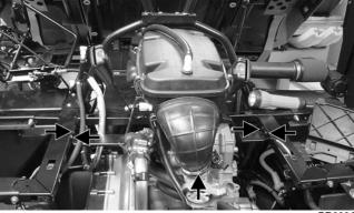
16. Connect the gasline hoses to the fuel rails making sure the "quick-disconnect" couplers properly lock onto the fuel injector rails.
