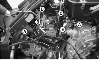
24. From the right side, connect the ECT sensor (A), IAT sensor (B), fuel pump/fuel gauge connector (C), rear ignition coil (D), and TPS connector (E).
