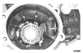
2. Using a propane torch, heat the area surrounding the needle bearing to soften the Loctite.
