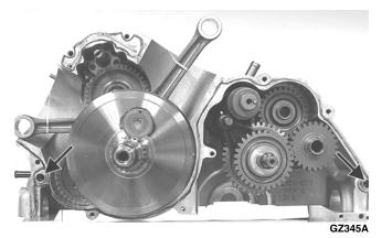
4. Carefully join the crankcase halves by placing the left-side crankcase onto the assembled right side. Secure with the cap screws (eight left side and one right side).
