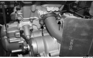
8. With a new grafoil gasket in the front cylinder head and a new grafoil seal on the exhaust pipe, install the front exhaust pipe and loosely secure with two cap screws.
