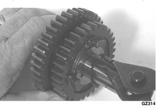
6. Remove the low driven gear. Account for a bearing, bushing, and thrust washer.
