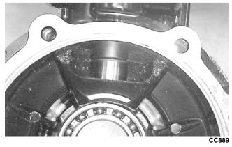
3. Install the pinion shaft and secure with the existing 48 mm lock collar. Tighten to 120 ft-lb.
