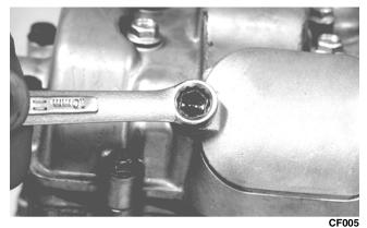
2. Rotate the crankshaft to the TDC position on the compression stroke of the front cylinder. The stamped "F" must be visible.
