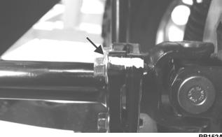
3. Remove the cap screws securing the propeller shaft flange to the yoke flange on the appropriate drive-line; then remove the propeller shaft.
