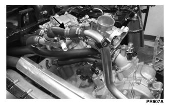
19. Remove the sheet metal screws securing the constant variable transmission (CVT) cooling duct to the frame; then loosen the hose clamps and remove the duct from the front elbow and CVT boot.
