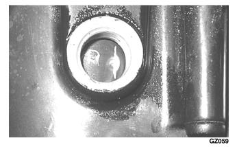
2. Remove the tappet covers on the cylinder being serviced. The tappets should not have pressure on them.
