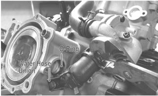
12. Remove the two nuts securing the cylinder to the crankcase.
