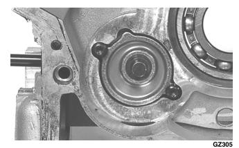
7. Remove the driveshaft (G); then remove the countershaft assembly (with shift forks) (H). Account for three flat washers on the countershaft.
