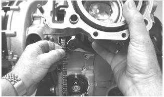
4. Loosely install the two nuts securing the cylinder to the crankcase.
