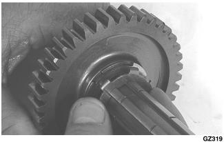
3. Remove the reverse driven gear dog.
