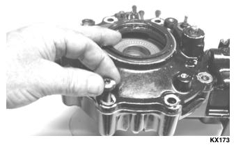
3. Using a plastic mallet, tap lightly to remove the differential cover. Account for an O-ring.
