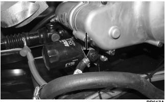
2. Using a suitable "T" fitting, connect Oil Pressure Test Kit to the oil fitting and hose. Tighten all clamps securely.
