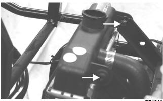
2. Connect the upper and lower coolant hoses to the radiator and secure with the appropriate hose clamps; then connect the cooling fan wire connector to the main harness.
