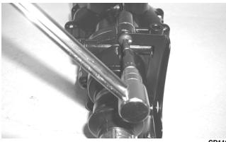
8. Install the proper shim onto the ring gear spider assembly making sure the chamfer side of the shim is facing toward the ring gear. Install the ring gear in the housing; then install the outside shim with the chamfer side of the shim toward the ring
