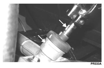
■NOTE: Any time steering components are disassembled, all connecting components should be marked for proper alignment during assembling.
