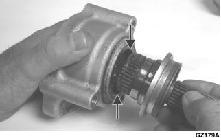
4. Install the clutch basket onto the input shaft and secure with the snap ring (flat side directed outward); then install the clutch pack into the basket.
