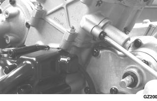
5. Using an awl, rotate the C-ring in its groove until it is out of the cylinder head; then remove the C-ring.
