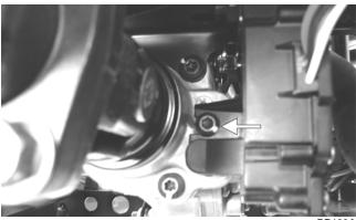
3. Remove the mounting cap screw from above the actuator on the suspension side.
