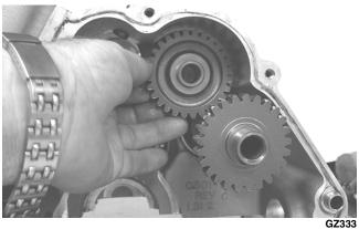
7. Install the gear shift shaft into the crankcase making sure the flat washer is in place on the gear shift position switch end and the bearing assembly on the gear shift stop end.
