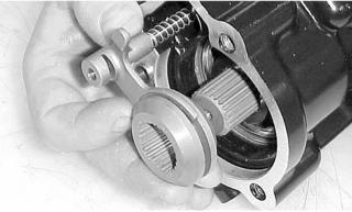
7. Place the input shaft assembly onto the housing; then secure with the existing cap screws. Tighten to 23 ft-lb.
