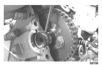
6. Bend the washer tabs down and remove the two cap screws securing the sprocket to the camshaft; then drop the sprocket off the camshaft.
