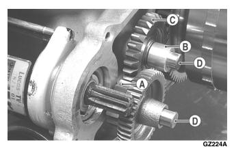
■NOTE: The starter is not serviceable and must be replaced as a complete assembly.
