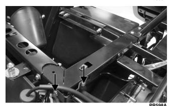
12. Remove the machine screw securing the throttle arm cover; then loosen the mounting nuts and disconnect the throttle cable from the throttle body.
