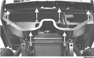
3. While lifting up on the front of the storage box, pry the rear center clear of the center dash mount and remove the storage box.
