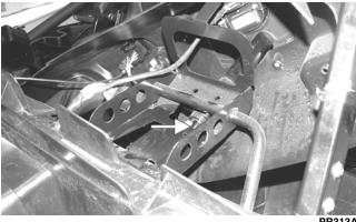
4. Match mark the upper steering shaft joint and the steering wheel shaft; then remove the steering wheel shaft. Account for the lower thrust-washer.
