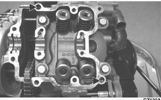
4. Remove the cap screw on the end of the tensioner; then using a screwdriver, turn the tensioner clockwise to remove the tension. Remove the two cap screws securing the tensioner adjuster assembly and remove the assembly. Account for a gasket.
