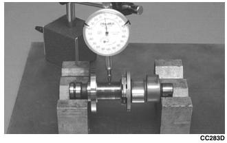
2. Rotate the camshaft and note runout; maximum tolerance must not exceed specifications.
