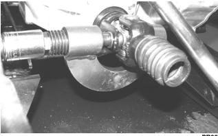
5. Check that the universal joint can be flexed freely without binding; then apply multi-purpose grease to the splines and install the propeller shaft noting the match marks made prior to removing. Tighten the cap screws to 40 ft-lb.
