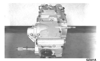
4. Remove one cap screw from the right-side crankcase and eight cap screws from the left-side crankcase; then using a rubber mallet, separate the crankcase halves leaving all components in the right-side case. Account for a thrust washer on the crankshaft and flat washers on gear shift shaft, countershaft, and reverse idler. Note the location of two alignment pins.
