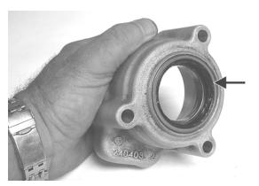
4. Remove the snap ring retaining the input bearing and using an appropriate bearing driver, press the bearing from the housing.
