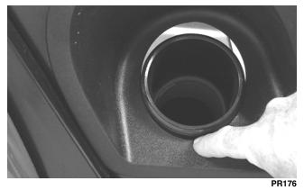
5. Secure the filler panel with four press-nuts; then tighten the hardware securing the hold-down straps (from steps 2-3) securely.
