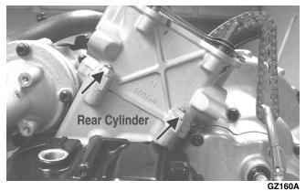
13. Lift the cylinder off the crankcase taking care not to allow the piston to drop against the crankcase. Account for the gasket and two alignment pins.
