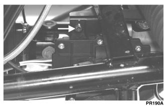
4. Loosen but do not remove the mounting cap screw at the front of the actuator; then slide the actuator to the rear enough to clear the slotted mounting tab and the selector shaft. Remove from the right side.
