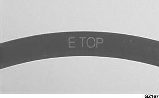
3. Install the first (unmarked) compression ring; then rotate the rings so the ring gaps are approximately 180° apart and orientated to the piston pin.
