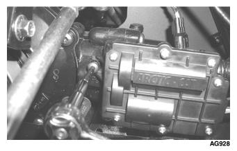
4. Loosen the front cap screw; then tighten the cap www.neromon.terptives.boffside.
