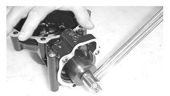
4. Place a punch on the edge of the lock collar in the oil gallery area; then using a hammer, stake the lock collar to ensure that the collar will remain securely tightened.
