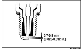
When installing the spark plugs, be sure to tighten it securely. A new spark plug should be tightened 1/2 turn once the washer contacts the cylinder head. A used spark plug should be tightened 1/8-1/4 turn once the washer contacts the cylinder head.
