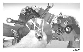
■NOTE: It will be necessary to rotate the crankshaft back and forth to engage the teeth of the oil pump and countershaft gears.
