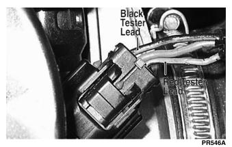
9. Select the DC Voltage position on the meter and turn the ignition switch to the ON position. The meter should read approximately 0.6 DC volts
