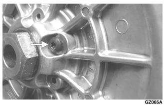
12. Place the V-belt into position on the driven pulley and over the front shaft.
