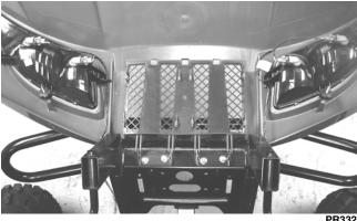
3. Connect the four headlight connectors; then secure the wires with two new nylon ties.
