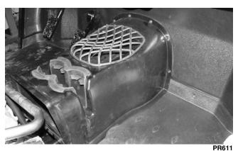
3. Remove the gas tank hold-down; then remove the gas tank cap.
