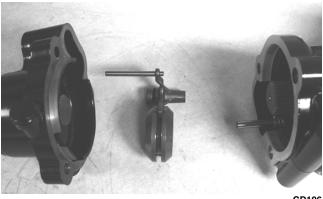
3. Remove the input shaft from the pinion housing.
