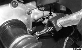
7. Install the cap screws securing the cable support to the caliper and tighten securely.
