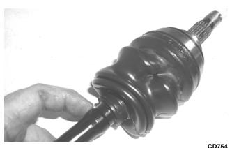
10. Using CV Boot Clamp Tool, secure both outside boot clamps.
