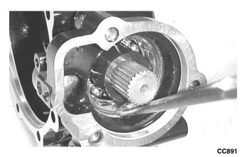
5. Install the pinion housing.
