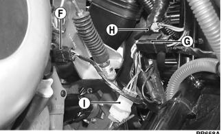
22. Route the engine harness through the shifter support brackets as marked during disassembly and secure with nylon cable ties.
