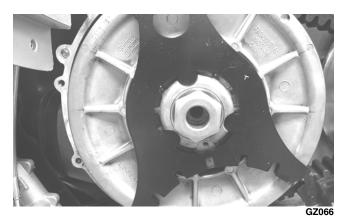
10. Slide the fixed drive face onto the clutch shaft.
