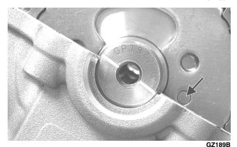
21. Seat the cam sprocket onto the camshaft making sure the alignment pin in the camshaft aligns with the smallest hole in the sprocket; then place the camshaft/sprocket assembly onto the cylinder ensuring the following.
