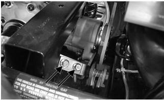
3. Remove the two cap screws securing the brake caliper to the gear case housing; then remove the caliper assembly from the vehicle.
