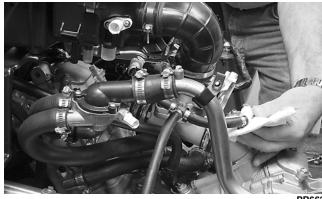
17. Install the shift support assembly and secure with four cap screws; then secure the upper coolant pipe support clamp to the shift support. Tighten the cap screws securely.
