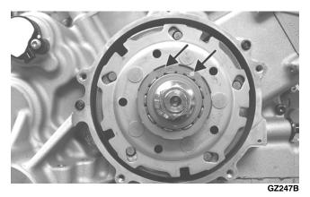
9. Using a hydraulic press, remove the clutch housing assembly from the clutch cover. Account for the left fixed drive spacer and an O-ring inside the fixed drive spacer.
