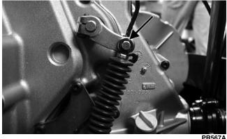
3. Loosen nuts (A) and (B) and adjust the cable housing to align the throttle cable end to the shift arm stud (C).
