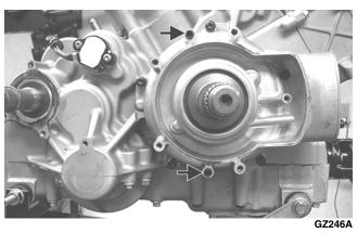
7. Remove the cap screws securing the clutch cover; then using a rubber mallet, carefully remove the cover. Account for two alignment pins.
