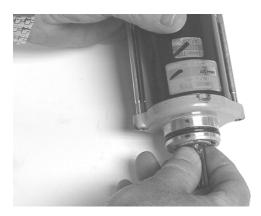
14. Using Crankshaft Seal Protector Tool, install the magneto cover using a new gasket and secure with the cap screws. Using the pattern shown, tighten to 8 ft-lb.
