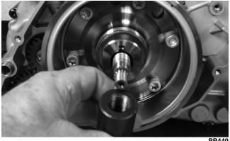
4. Install Magneto Rotor Remover Set and loosen the rotor/flywheel; then remove the crankshaft protector and rotor/flywheel from the crankshaft. Account for the flywheel key.
