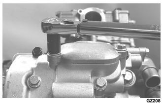
38. If removed, install the spark plugs. Tighten securely.
