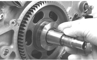
5. With the flywheel key removed, remove the starter
