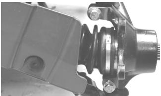
7. Install the tie rod end and secure with the nut (coated with red Loctite #271). Tighten to 30 ft-lb; then install a new cotter pin and spread the pin to secure the nut.
