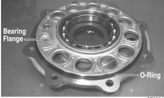
11. Making sure the O-ring is properly positioned on the differential housing cover assembly, install the cover with existing cap screws (coated with green Loctite #609). Account for the ID tag. Tighten the cap screws to 23 ft-lb.
