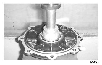
■NOTE: Prior to installing the seal, apply grease to the seal outside diameter.
