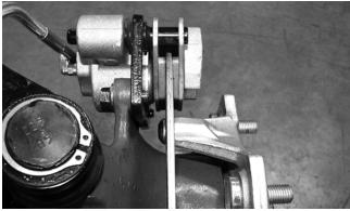
2. Install the A-arm assemblies into the frame mounts and secure with the cap screws. Only finger-tighten at this time.
