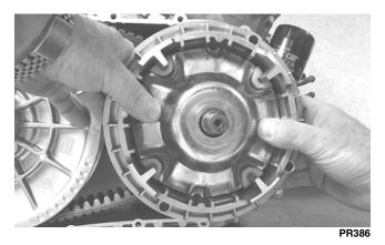
■NOTE: At this point, the cap screw can be removed from between the driven pulley faces.
