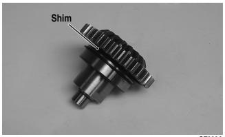
2. If backlash measurement is more than specified, remove an existing shim, measure it, and install a thicker shim.
