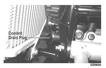
■NOTE: Always use a large container and have sufficient floor drying material available when draining the coolant in case of coolant spillage.
