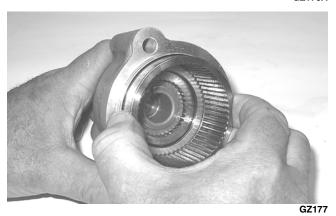
3. Remove the input shaft from the input housing; then remove the oil seal.
