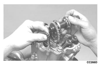
■NOTE: Loop the chain over the cylinder head and secure it to keep it from falling into the crankcase.
