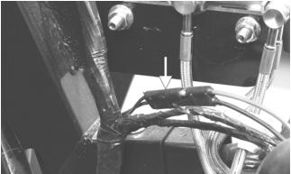
5. Remove the two shoulder bolts and nuts securing the radiator to the frame; then disconnect the upper and lower coolant hoses.
