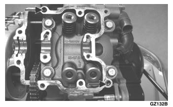
9. Remove the cylinder head from the cylinder, remove the gasket, and account for two alignment pins; then remove the cam chain guide.
