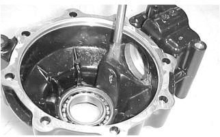
3. Using a flat-nosed punch, drive the bearing out of the housing.
