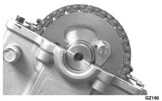
24. Rotate the crankshaft until the second cap screw securing the sprocket to the camshaft can be installed; then install the cap screw (threads coated with red Loctite #271) and tighten to 11 ft-lb. Bend the tab to secure the cap screw.
