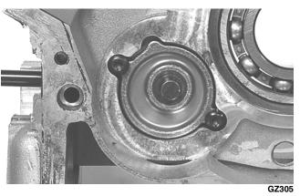
2. Install a flat washer, drive pin, and drive gear onto the oil pump shaft; then secure with a snap ring (flat-side away from the gear).
