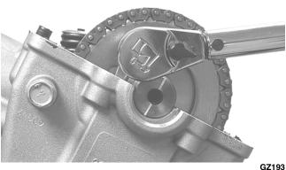
18. Rotate the crankshaft until the first cap screw (from step 16) can be tightened; then tighten to 11 ft-lb. Bend the tab to secure the cap screw.
