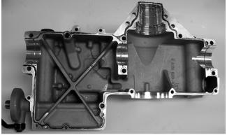
8. Carefully place the lower crankcase cover onto the joined crankcase halves; then secure with the cap screws. Tighten the 6 mm cap screws to 8 ft-lb and the 8 mm cap screws to 20 ft-lb.
