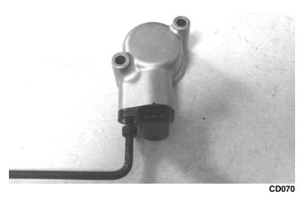
3. Install the new speed sensor into the housing with new O-ring lightly coated with multi-purpose grease; then secure the sensor with the Allen-head cap screw (threads coated with blue Loctite #242). Tighten securely.
