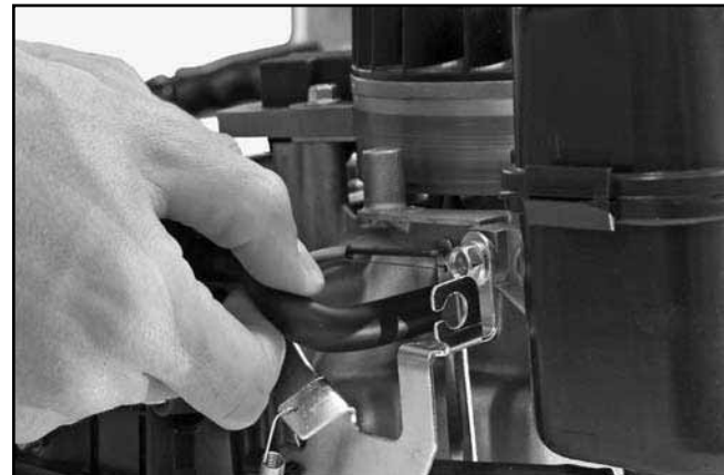
Figure 8-11. Detaching Breather Hose.
