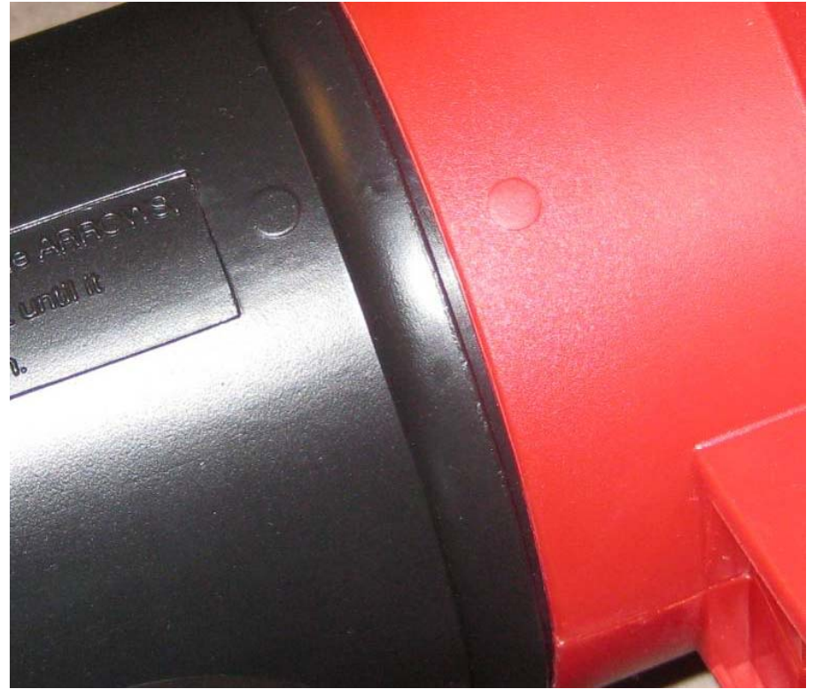
Incorrect – not locked
