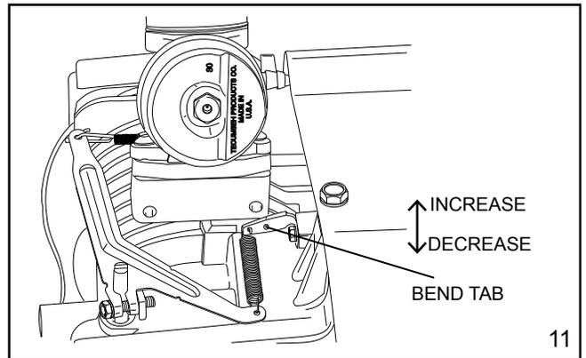
R.P.M. adjustment of fixed speed models is done by bending the tab as shown.
