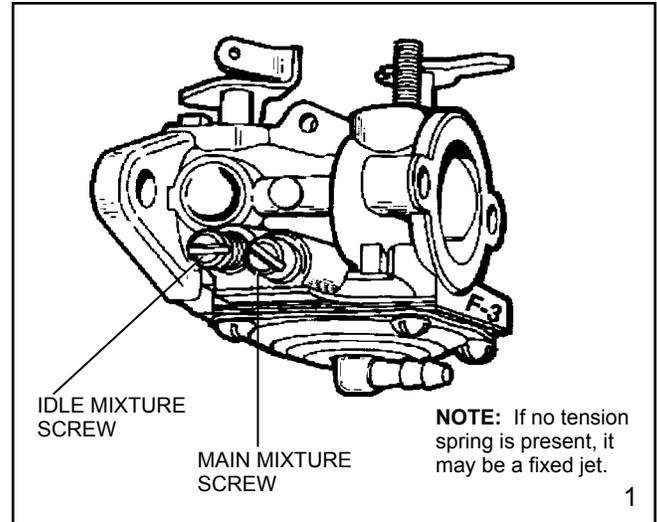
Start the engine and let it warm up for approximately 3-5 minutes. Do not adjust the carburetor when the engine is cold.
