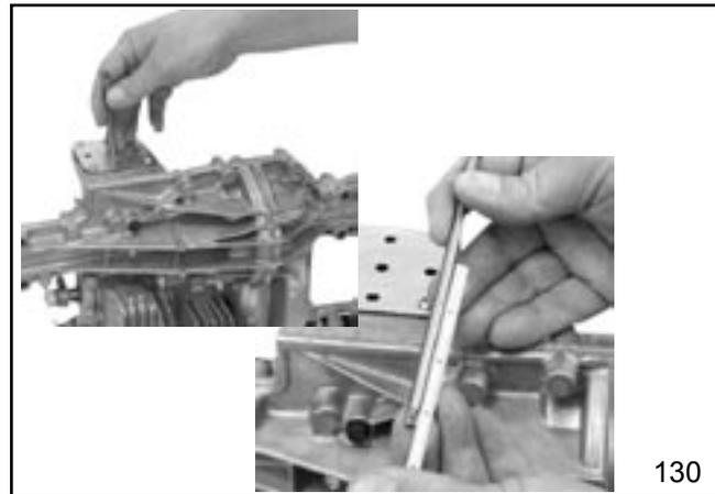
3. If the measurement is beyond the dimensions listed, the next step is to remove the transaxle from the frame. Then thoroughly wash and blow dry the bellows cover area as shown. Remove all impurities before removing the bellows cover.
