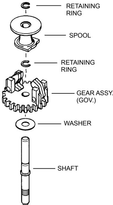
\* As of August 1992, all small frame engines, including VLV40-6.75, use a retainerless shaft. Service replacement shafts will be retainerless for all small frame and VLV engines.
