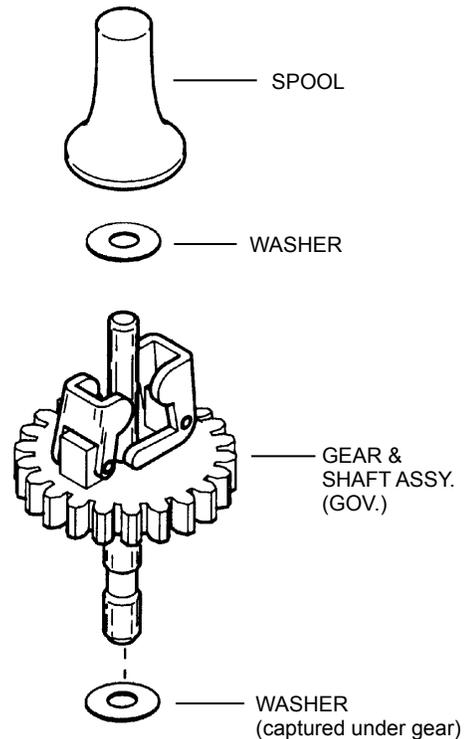
**NOTE:** On models OHV13.5-17, the spacer is cast as part of the governor gear with the washer placed below the gear assembly.
