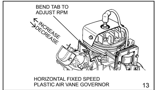
To disassemble, remove choke shutter with needle-nose pliers; the vane assembly may then be removed from the carburetor.
