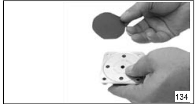
When reusing the old cover it is difficult to seal all five holes. One other way to compress the bellows is to invert the inside tab and place a slip knot made from thin string over it. Push the end of the bellows back to its original form and pull the string through the cover. When step six is complete, cut the string.
