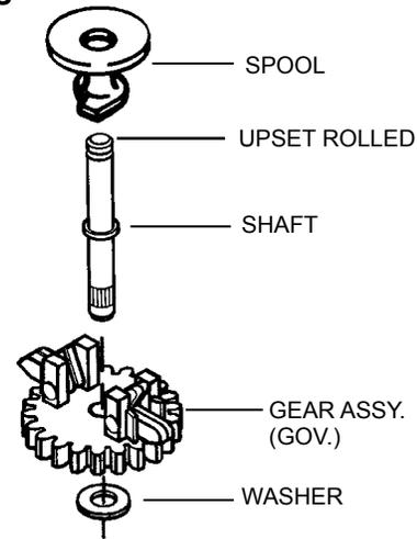
**NOTE:** Gear assembly must have .010 - .020 (.25 - .50 mm) end play after shaft is installed into flange.
