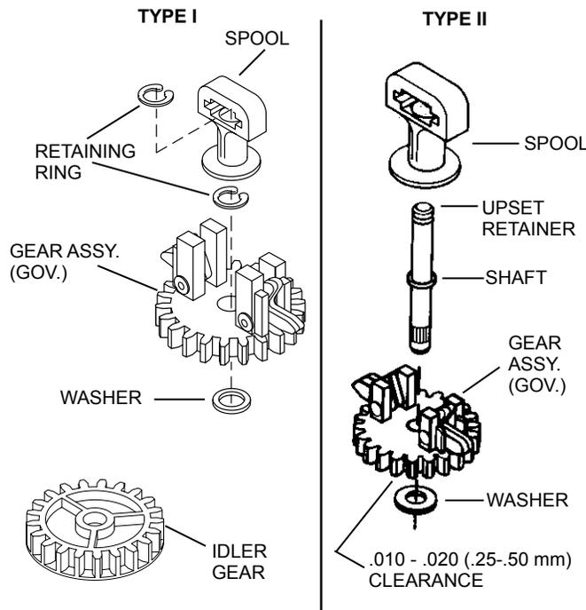
**NOTE:** Gear assembly must have .010 - .020 (.25 - .50 mm) end play after shaft is installed into flange.
