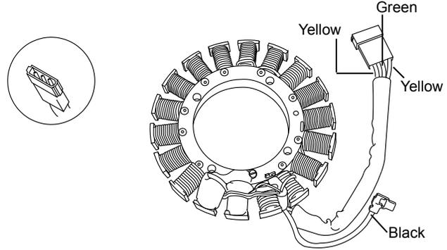
\* Uses regulator/rectifier 610996 or 610907A; depending on spec. number; an open circuit D.C. voltage check cannot be made.
