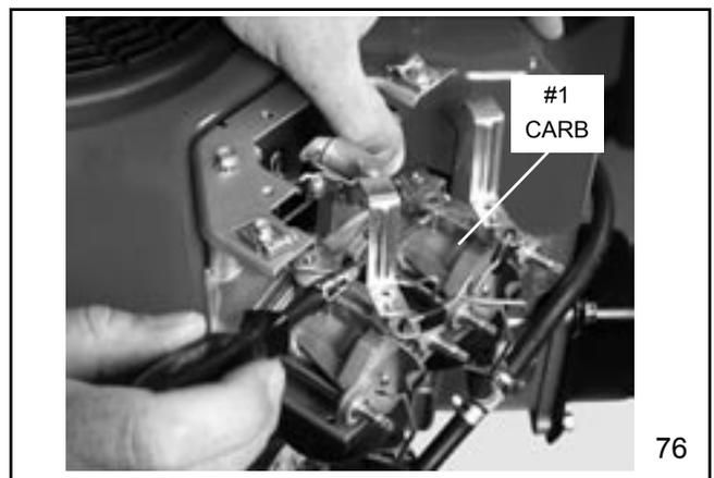
6. Connect both carburetors by attaching the link and link connector bushing clip to the # 1 carburetor.
