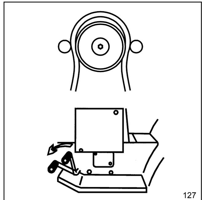
With clutch disengaged, it is very important that the belt blossoms away from the engine pulley. Belt must stop turning before transaxle shifting can occur.
