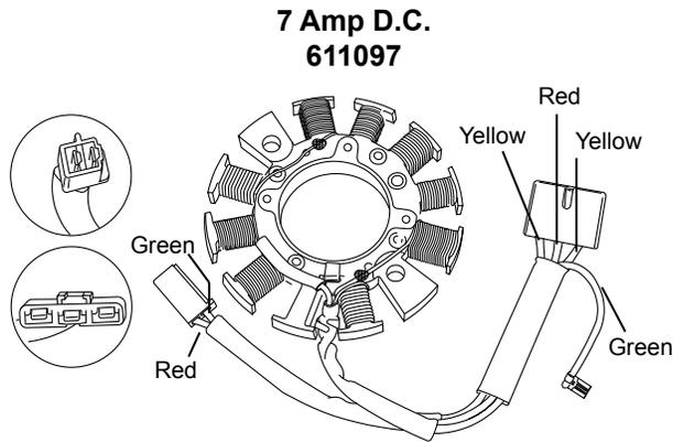
\* Uses regulator/rectifier 611098; an open circuit D.C. voltage check cannot be made.
