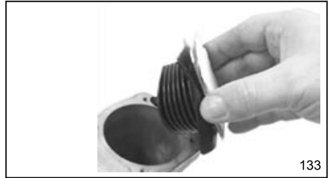
This can also be done by using a refrigerator magnet cut to cover the hole. (The new bellows cover comes with only one hole in the center and seals very easily).
