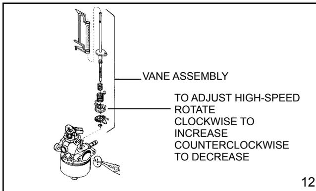
Rotate sleeve clockwise to increase R.P.M., counterclockwise to decrease R.P.M.
