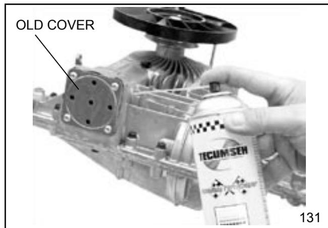
4. Turn the unit so that the bellows chamber faces up as shown. Remove the bellows cover screws using Tecumseh tool **part #670332** torx bit. Then add oil **part #730228A** until the amount present measures 1-29/32 inch (48.41 mm) from the top edge of the bellows housing.
