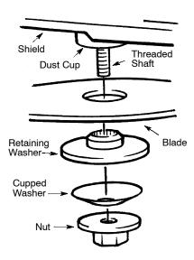
**NOTE:** Make sure all parts are in place as illustrated, and the blade is sandwiched between the dust cup and the retaining washer. There should be no space between the blade and the dust cup or the retaining washer.
